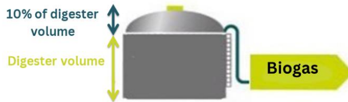
Figure 14. Scheme of the biodigester
