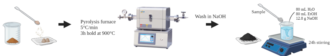
Figure 2.6: First pyrolysis and wash in NaOH
