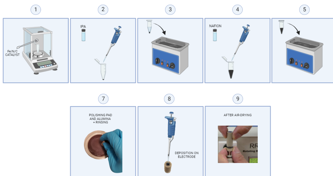
Figure 2.18: Preparation of ink and rotating disk electrode
