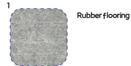
Rubber flooring is highly durable and well-suited for high-traffic areas. Its softer composition helps reduce noise levels, making it ideal for spaces where sound absorption is important, such as large open areas prone to echoes.
