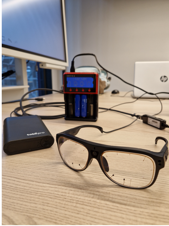
Figure 2.8: Tobii Glasses 3 setup and his additional devices
