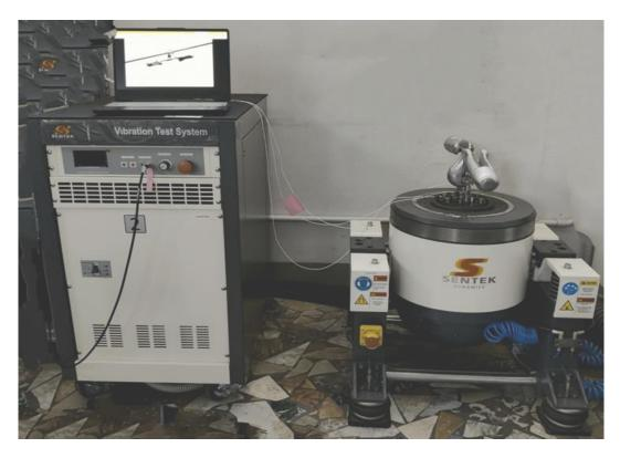
Figure 2.3. Experimental setup for Stockbridge analysis (Lab)
