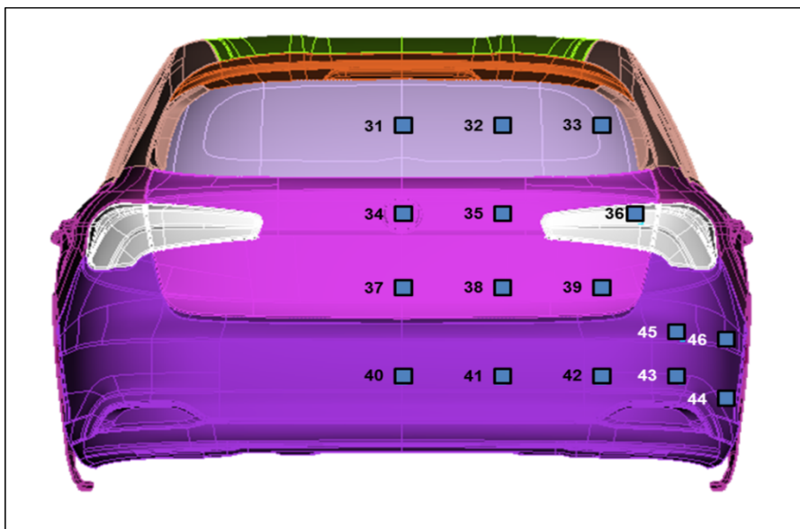
Figure 4.20: Pressure sensors position - 6
