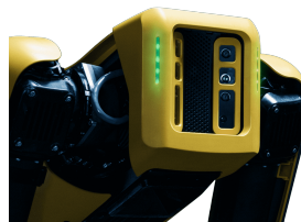
Figure 4.1: Front fisheye cameras of Spot
