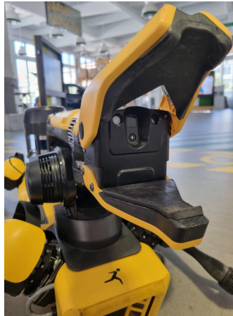
Figure 4.3: Spot Arm Gripper camera
