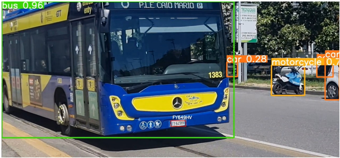
Figure 3.8: License place recognition with YOLOv8 of a frame from a video taken with Spot
