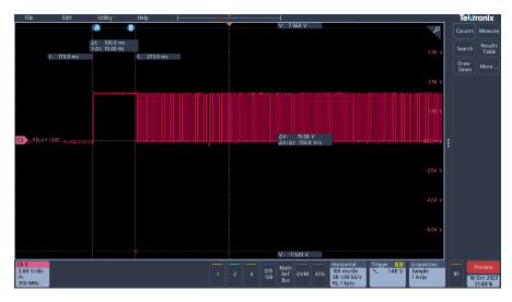
Figure 8.4: Channel 3 shows the peak and hold signal
