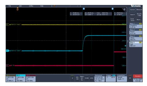
Figure 7.8: Channel 1 (yellow line) shows the DC Fault signal not considered in this test; Channel 2 (blue line) shows the AC Fault signal; Channel 3 (red line) shows the relay feedback not considered in this test
