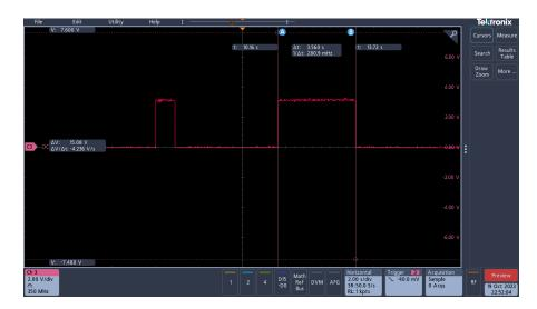
Figure 7.7: Channel 3 (Red line) is the DC Fault signal. On the left side, the fault time is lower than 2 s, while on the right the time is measured and is equal to 3.56 s
