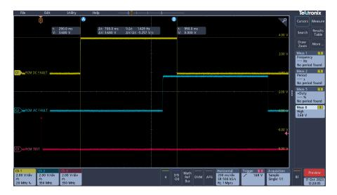
**Figure 7.9:** Channel 1 (yellow line) shows the DC Fault signal; Channel 2 (blue line) shows the AC Fault signal; Channel 3 (red line) shows the input test signal
