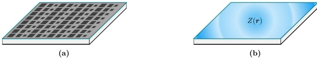
**Figure 1.3:** (a) Actual metasurface and (b) homogenized metasurface with the surface impedance distribution.
