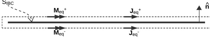
**Figure 3.1:** Graphical application of the Equivalence theorem. The dashed line represents the volume containing the sources.
