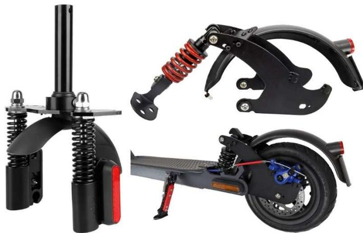
*Figure 3.11. Examples of typical front and rear electric scooter suspension systems*
