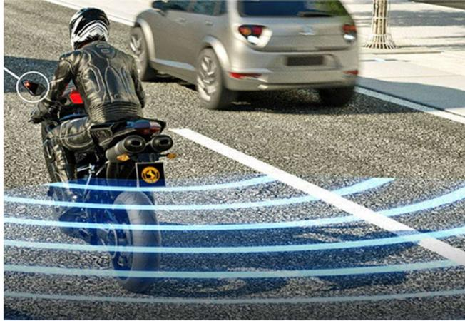
*Figure 1.8. Illustration of an ADAS system employed on a two-wheeled vehicle (in the figure, the Blind spot detection warns the rider with a display in the rear-view mirror)*
