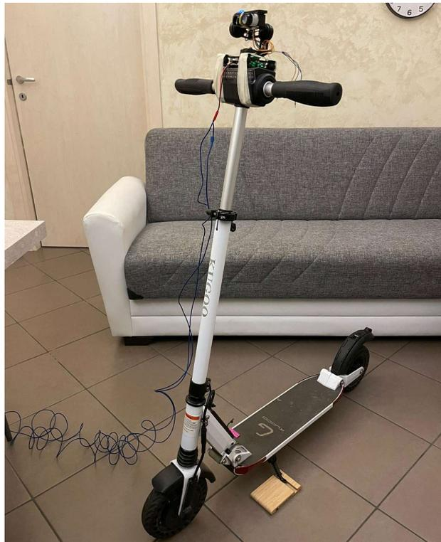
*Figure 3.1. Complete sensing system installed on the electric scooter*
