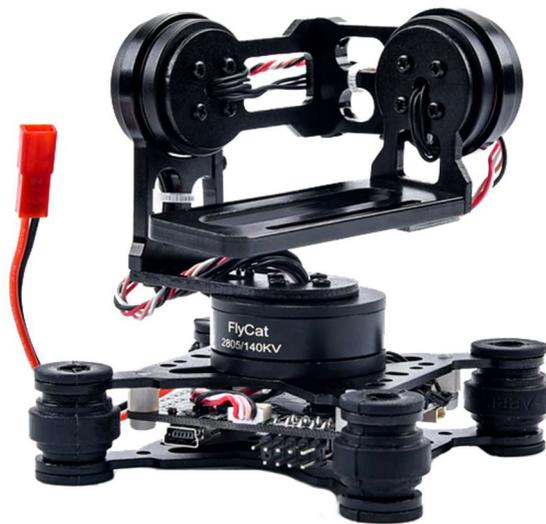
*Figure 2.3. Storm32bgc, brushless gimbals with 3 axes based on a STM32 32-bit microcontroller*
