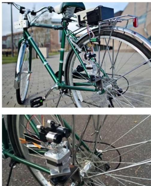
*Figure 1.9. Bicycle equipped with an active tracking device*
