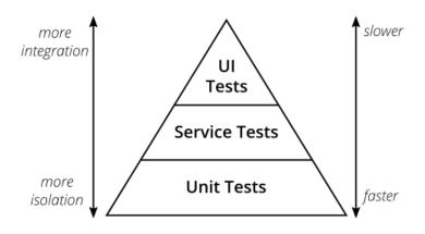
Figure 2.1: The Test Pyramid<sup>1</sup>
