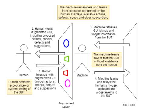
Figure 2.3: Augmented Testing Workflow
