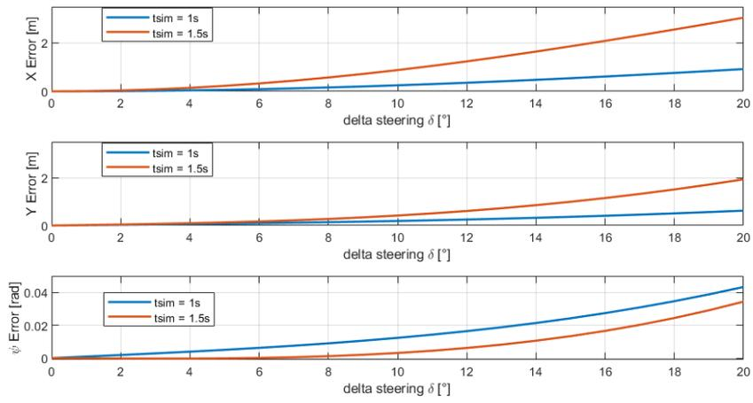
Figure 2.11: Prediction error over 1 second and 1.5 seconds at constant inputs.
