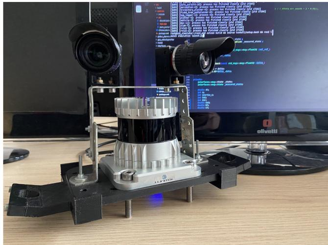
**Figure 1.4:** Lidar and Camera system of the VaLentina prototype.
