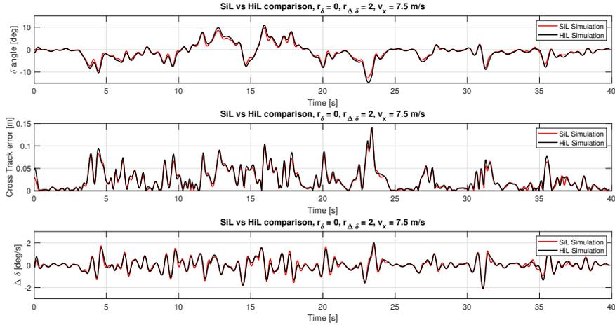
**Figure 4.7:** Comparison between SiL simulation and HiL simulation.
