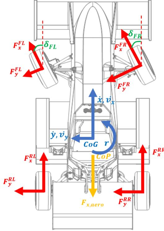
**Figure 2.3:** Forces acting on the vehicle, overhead view.
