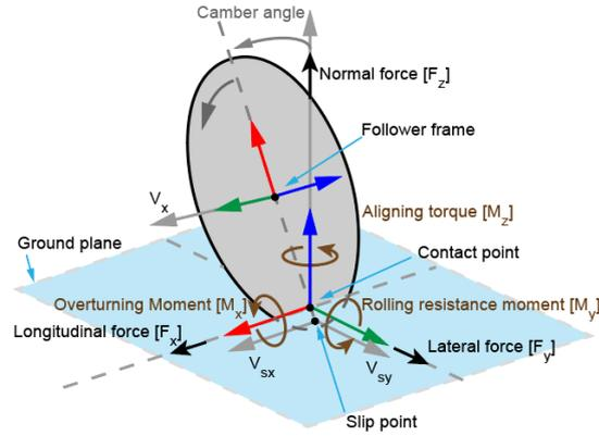
Figure 2.1:  $R_w$  reference frame following ISO sign convention.
