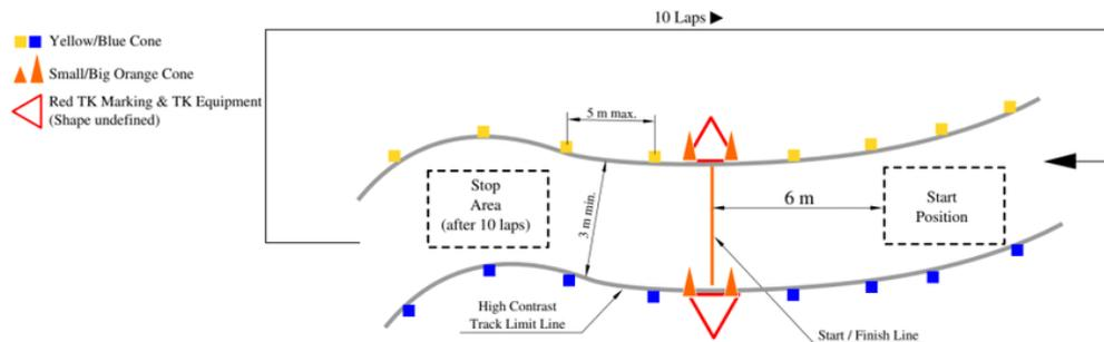
**Figure 1.2:** FSAE DV track cones layout.
