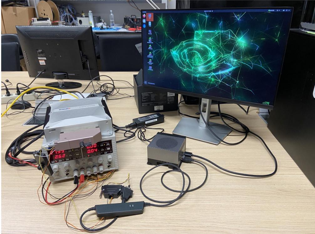
**Figure 4.6:** HiL setup: the NVIDIA Jetson AGX Orin (in the middle) communicating with the dSPACE MicroAutoBox III (on the left) via Kvaser Leaf Light V2 (on the bottom).
