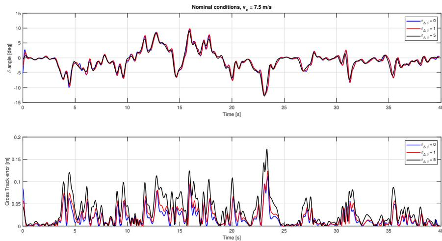
**Figure 4.3:** Effects of  $r_{\Delta\delta}$  on the steering angle  $\delta$  and on the performance parameter Cross Track error in nominal conditions.
