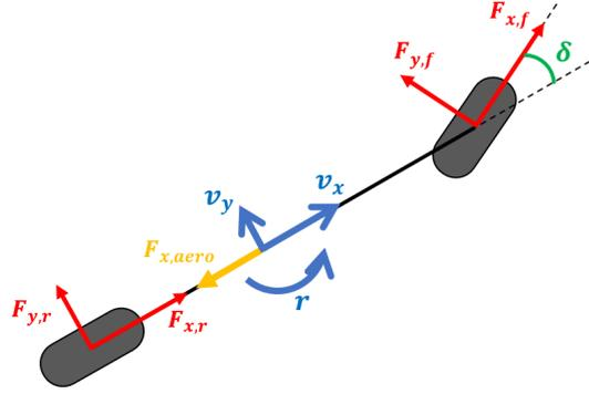
Figure 2.10: Bicycle model with acting forces.
