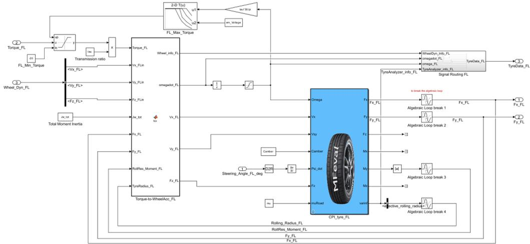
**Figure 2.5:** Wheel subsystem simulation model developed on MATLAB<sup>®</sup> Simulink.
