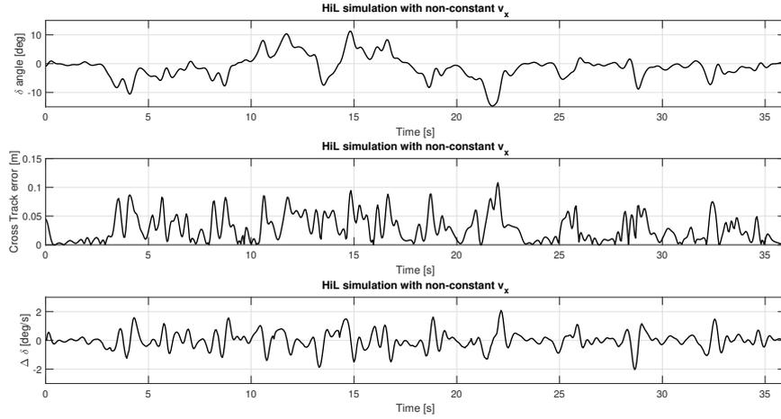
**Figure 4.8:** Complete HiL Simulation including longitudinal and lateral control, MPC performances.
