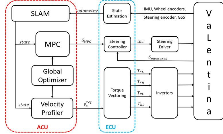
**Figure 3.1:** High level overview of the control scheme in which the MPC will be deployed.
