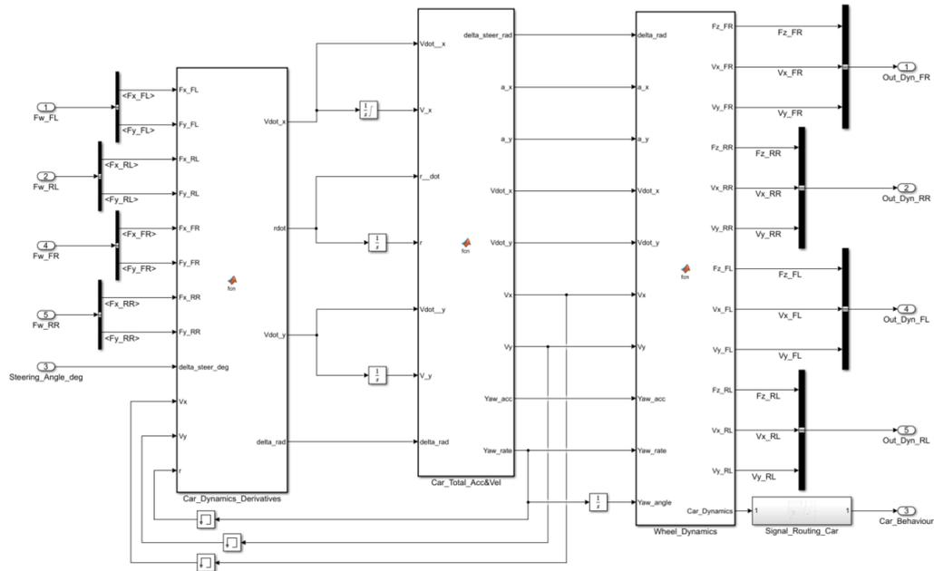
**Figure 2.6:** Chassis subsystem simulation model developed on MATLAB<sup>®</sup> Simulink.
