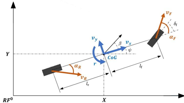
**Figure 2.9:** Bicycle Model representation in  $RF^0$ .
