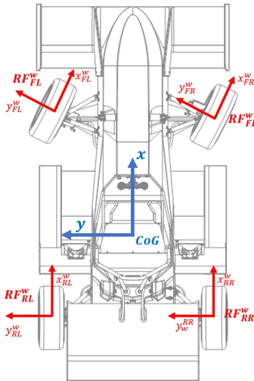
Figure 2.2: Reference Frames:  $RF^1$  and  $RF^w$ .
