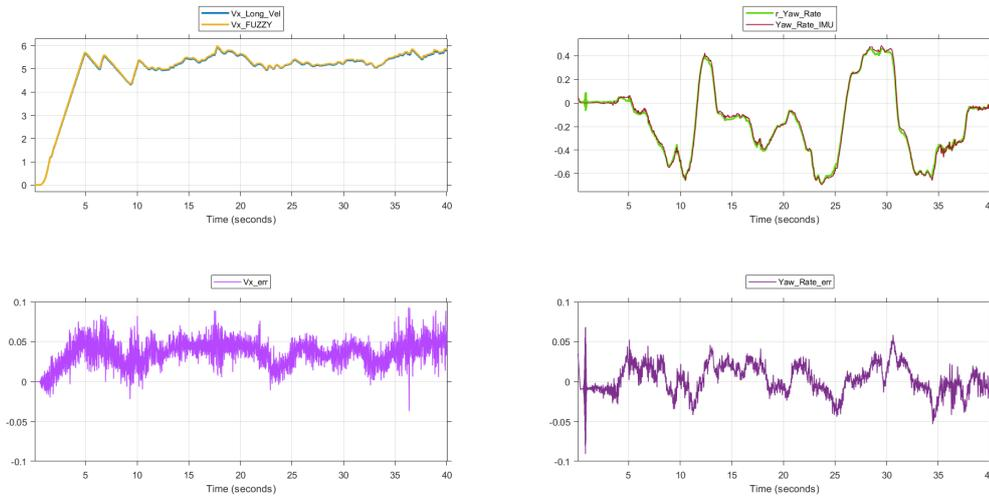
**Figure 2.8:** Data comparison between the simulation model and track-tests data.
