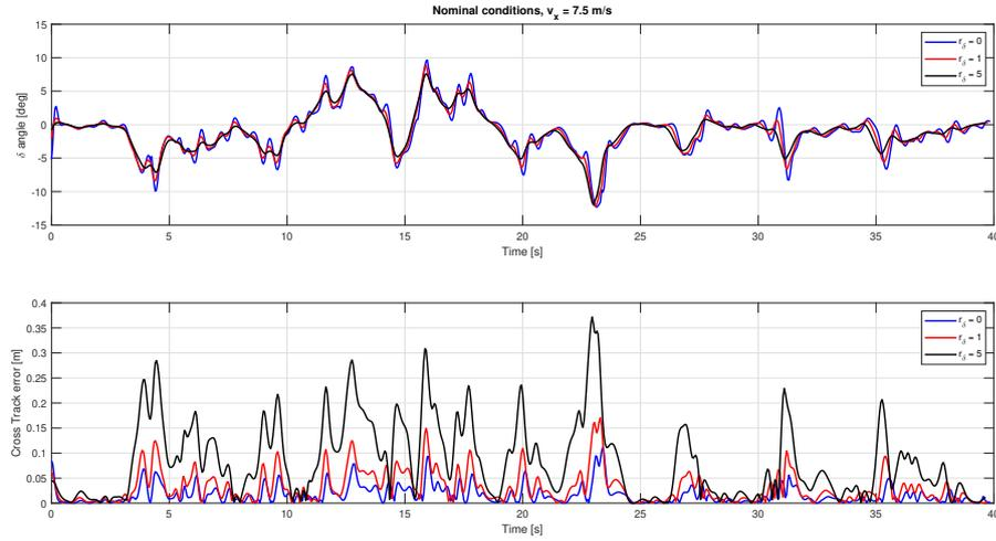
**Figure 4.2:** Effects of  $r_\delta$  on the control input and on the performance parameter Cross Track error in nominal conditions.
