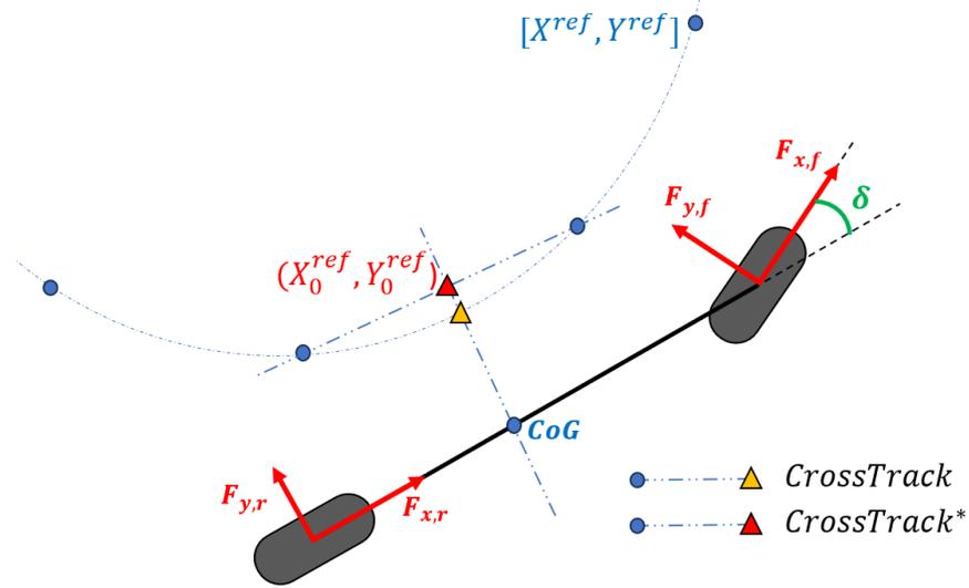
**Figure 3.2:** Cross Track Error between the vehicle and the reference trajectory
