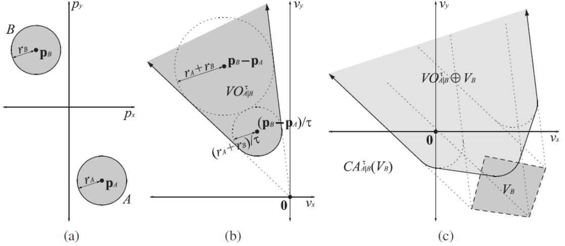
**Figure 4.3:** (a) A configuration of two agents. (b) The velocity obstacle  $VO_{A/B}^\tau$ . (c) The set of collision-avoiding velocities  $CA_{A/B}^\tau(V_B)$  for agent A given that B selects its velocities from some set  $V_B$  [9].
