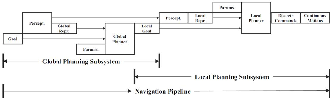
Figure 2.2: Navigation pipeline[13]
