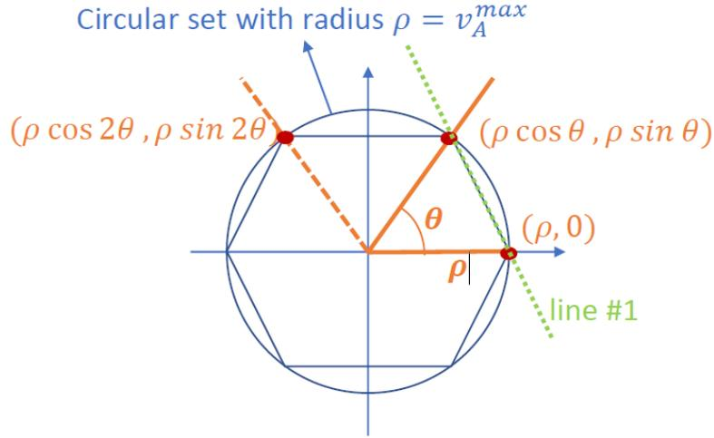
**Figure 4.6:** A scheme explicating the approximation of a circular set by means of  $n_{edg}$  half-planes.
