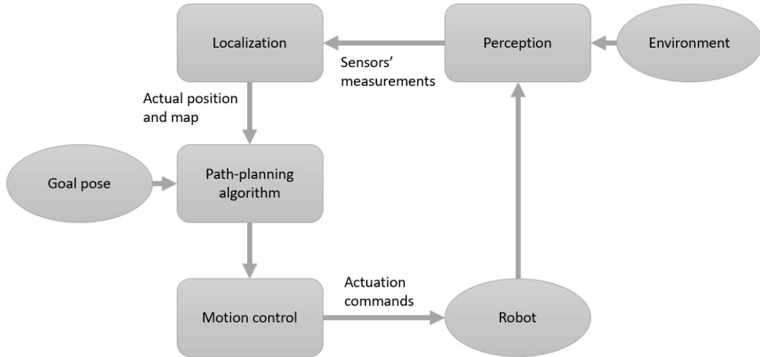
**Figure 2.1:** Robot navigation scheme
