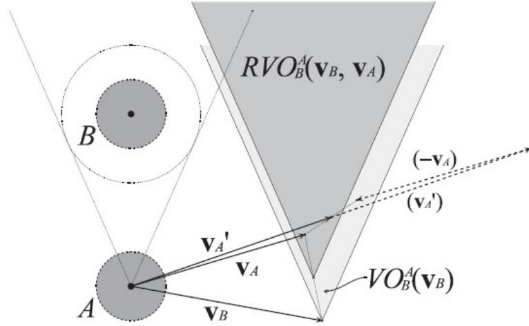
**Figure 4.2:** The Reciprocal Velocity Obstacle  $RVO_B^A(\mathbf{v}_B, \mathbf{v}_A)$  of agent B to agent A [32].
