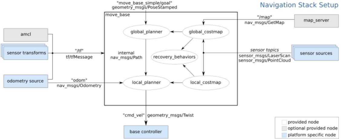
Figure 5.2: `move_base` package schematic overview [67].
