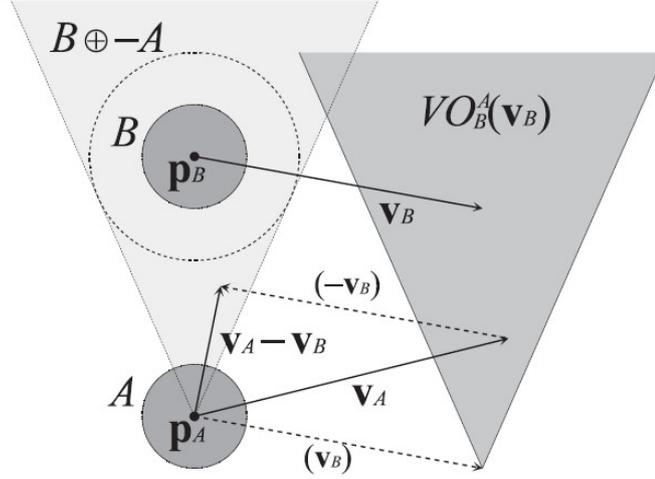
**Figure 4.1:** The Velocity Obstacle  $VO_B^A(\mathbf{v}_B)$  of a disc-shaped obstacle B to a disc-shaped agent A [32].
