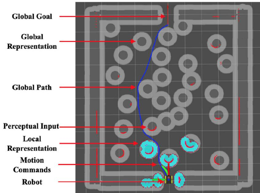
Figure 2.3: Navigation elements represented into a sample map[13]
