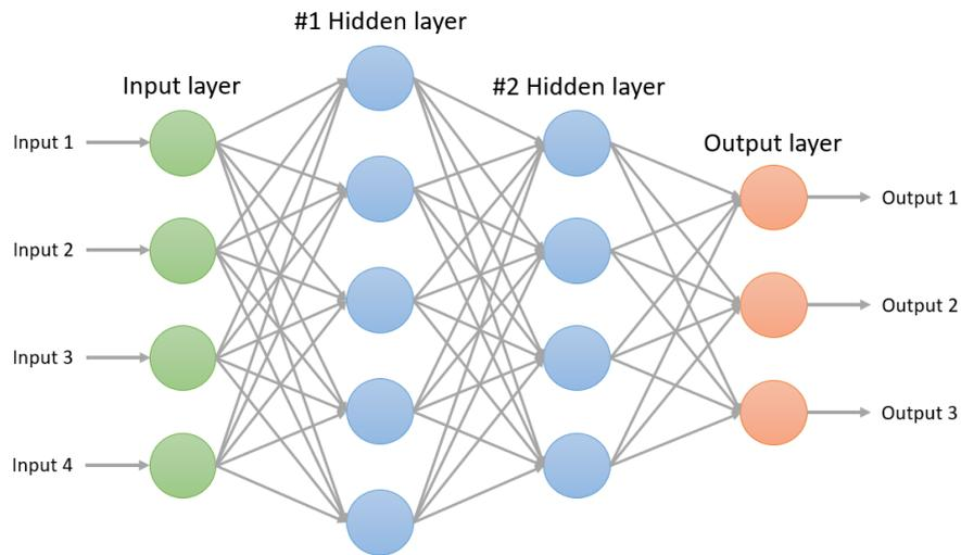
**Figure 5.6:** Representation of a simplified Fully-connected Neural Network (FCNN). It is composed by four input neurons, two hidden layers of five and three neurons and three output neurons.
