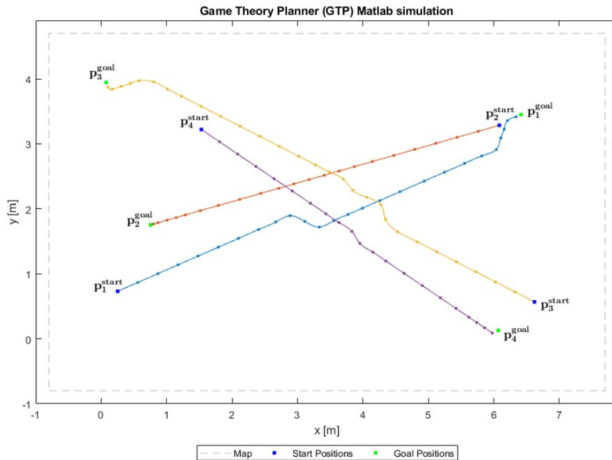
**Figure 6.1:** Generated trajectories obtained considering four agents moving with the proposed Game Theory prediction model.
