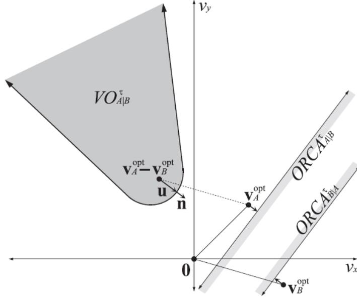
**Figure 4.4:** Geometrical construction of  $\text{ORCA}_{A/B}^{\tau}$  and  $\text{ORCA}_{B/A}^{\tau}$  [9].
