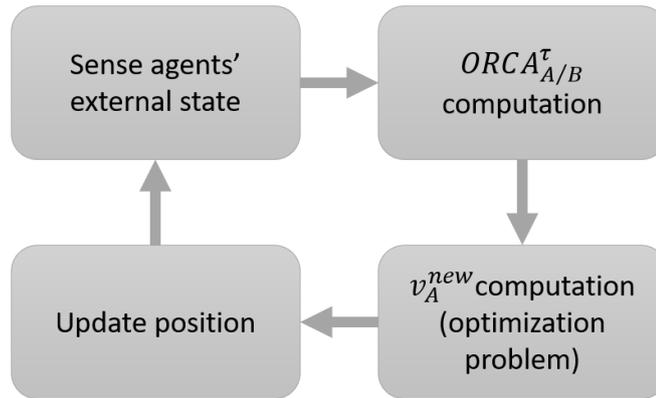
**Figure 4.5:** A schematic overview of the sensing-acting loop performed by the actor during a step [9].
