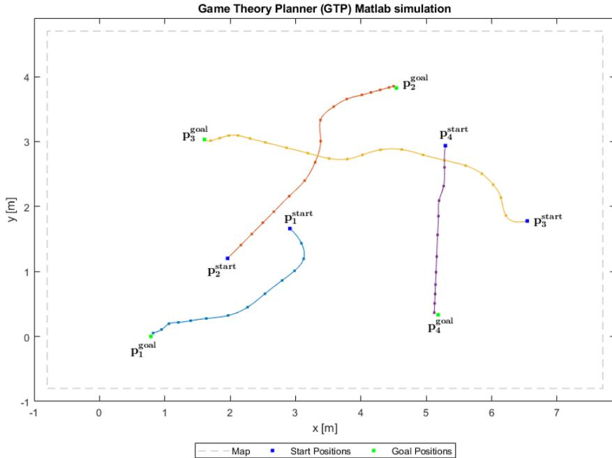
**Figure 6.3:** Generated trajectories obtained considering four agents moving and seven possible actions.
