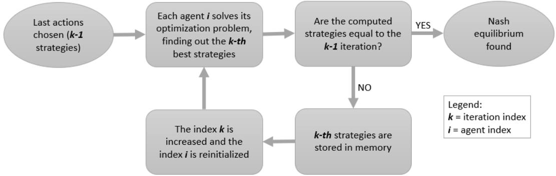
**Figure 4.7:** Simple scheme explaining the Sequential Best Response Approach applied in our context.
