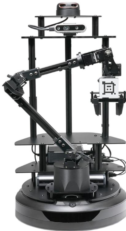
**Figure 1.1:** Locobot WX250s from Trossen Robotics[10]
