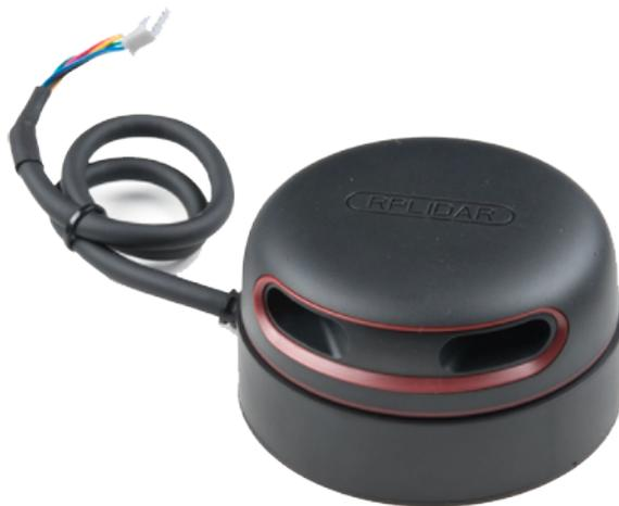
**Figure 5.10:** RPLIDAR A2M8 [10].
