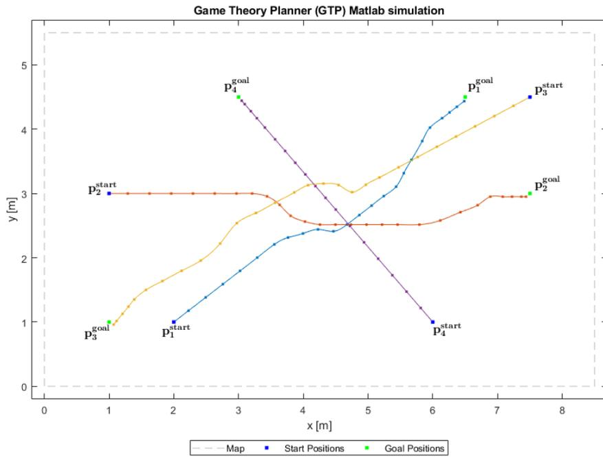
**Figure 6.4:** Generated trajectories obtained considering four agents moving and nine possible actions.
