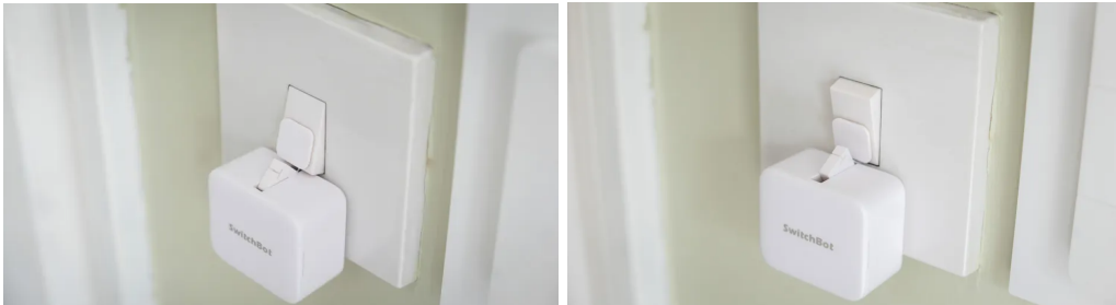
Figure 4.3: Use SwitchBot to turn on a light
