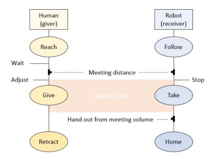
Figure 1.5: Structure of hand over task for human and robot. Reprinted from [19].
