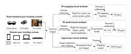
Figure 2.2: Gaze estimation methods . Reprinted from [30].
