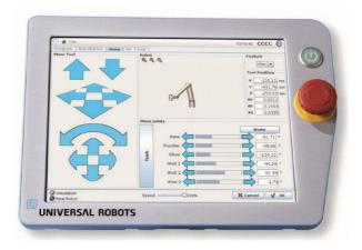
Figure 4.3: The teach pendant of the UR5 robot. Reprinted from [50]
