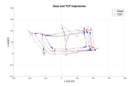
**Figure 5.6:** Original gaze signal case. Trajectories of gaze (in red) and of TCP (in blue) in xy plane.
