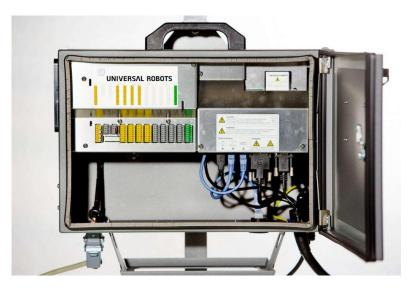
Figure 4.2: The control unit components of the UR5.
