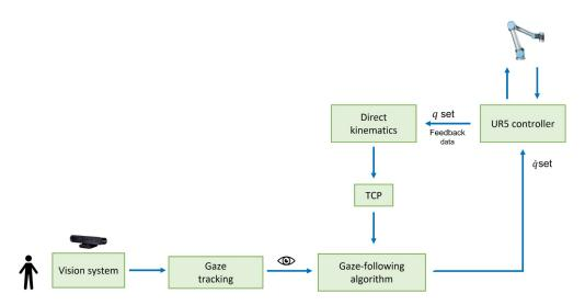
Figure 5.1: Scheme of the control loop adopted to manage the UR5 robot movements.
