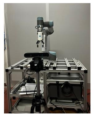
**Figure 5.4**: Experimental setup: UR5 manipulator fixed in the workbench and the Astra Orbbec camera in front of it
