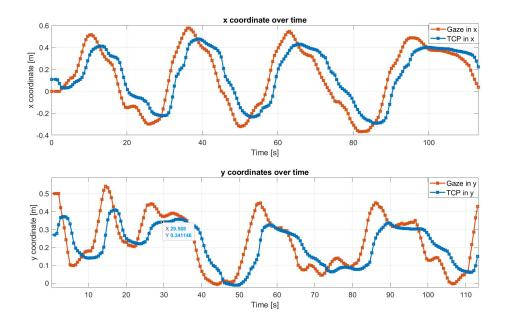
**Figure 5.13**: Filtered gaze signal case (filter size 10) of x and y trajectories over time. In red the gaze trajectory and in blue the TCP trajectory.
