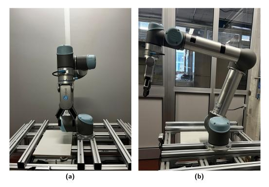
**Figure 5.5**: Home position configuration set for the UR5 robot. (a) Frontal view (b) Lateral view
