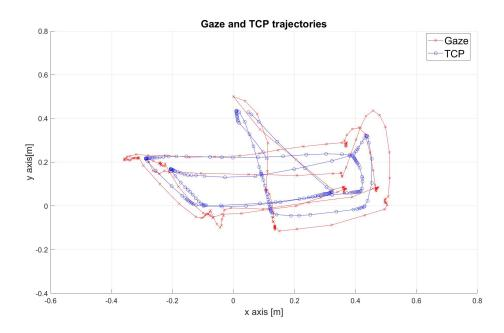
**Figure 5.9**: Filtered gaze signal case (filter size 5). Trajectories of gaze (in red) and of TCP (in blue) in xy plane.
