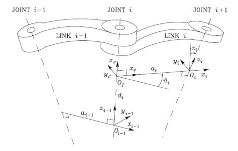
Figure 4.6: Standard Denavit Hartenberg convention representation. Reprinted from [53]
