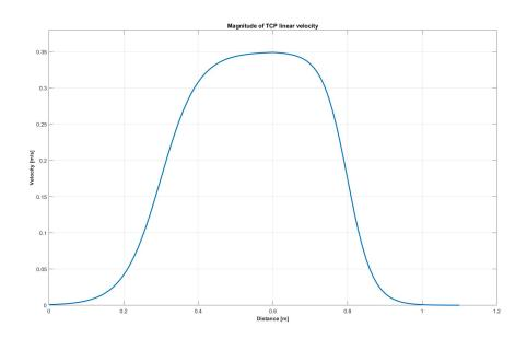
**Figure 5.2**: TCP linear velocity with respect to the distance between the gaze point and the TCP. The maximum TCP velocity was set to 0.35 m/s.
