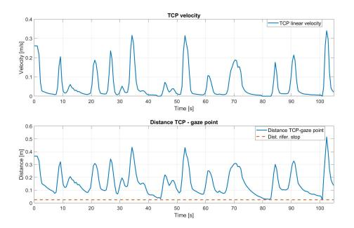
**Figure 5.11:** Filtered gaze signal case (filter size 5).Norm of the TCP linear velocity over time and related distance gaze point-TCP.
