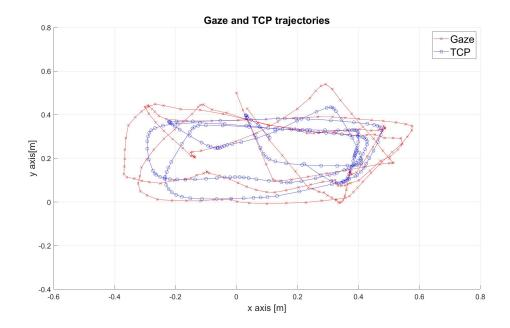
**Figure 5.12:** Filtered gaze signal case (filter size 10).Trajectories of gaze (in red), and of TCP (in blue) in xy plane.
