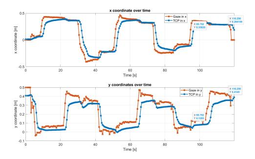
**Figure 5.7:** Original gaze signal case. x and y trajectories over time. In red the gaze trajectory and in blue the TCP trajectory.
