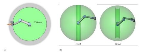
**Figure 4.5: (a)** Maximum, 850 mm, and recommended workspace, 750 mm, of UR5. **(b)** Cylindrical volume of 200 mm above and below the robot base. Moving the tool close to the cylindrical volume should be avoided. Reprinted from [49]
