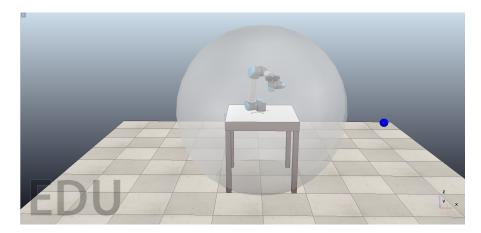
**Figure 5.3**: CoppeliaSim scene of robot UR5 positioned in the workbench in home configuration and its workspace area.
