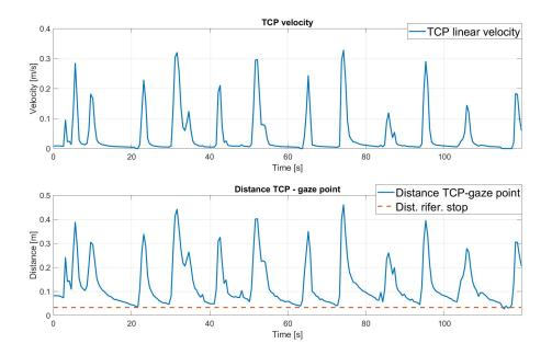
**Figure 5.8**: Original gaze signal case. Norm of the TCP linear velocity over time and related distance gaze point-TCP.
