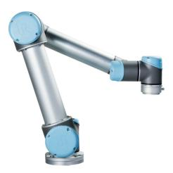
Figure 4.1: UR5 robot from Universal Robot. Reprinted from [49]
