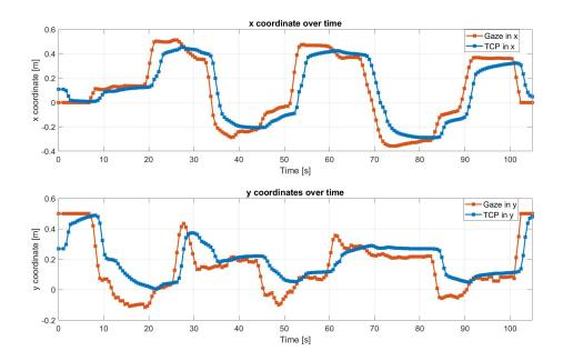
**Figure 5.10**: Filtered gaze signal case (filter size 5) of x and y trajectories over time. In red the gaze trajectory and in blue the TCP trajectory.
