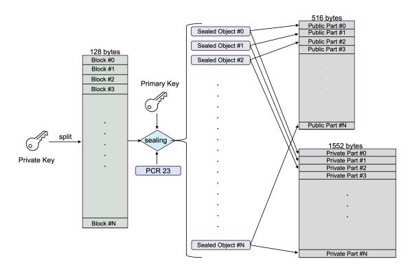
Figure 5.1. Sealing process overview
