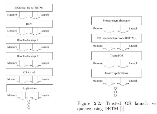
Figure 2.1. SRTM boot chain rooted in the BIOS boot block [1]
