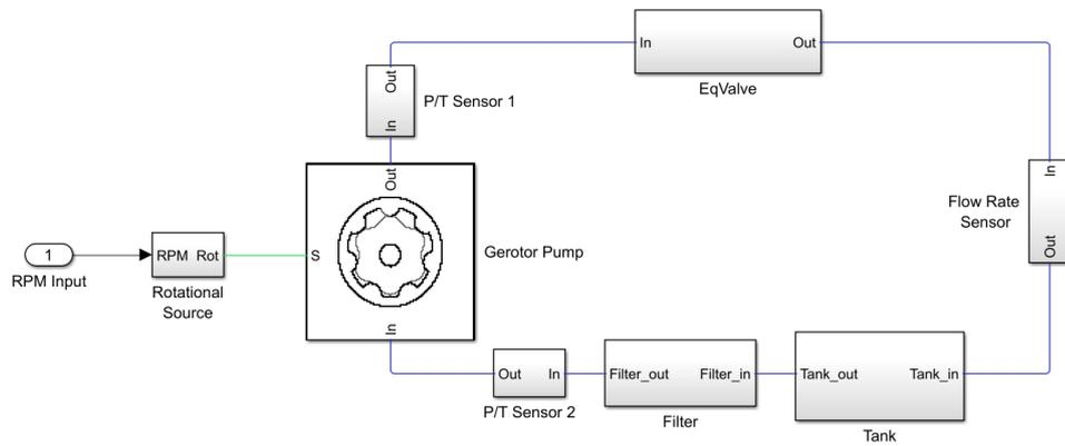
**Figure 5.7:** Final Model Simulink representation. Integrating the gerotor model with the final model architecture.
