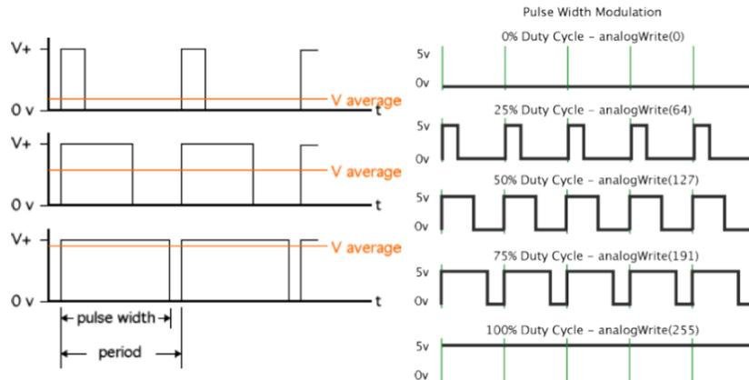
**Figure 6.1:** Pulse Width and Duty Cycle variation. Note: Adapted from *Design-Build-Code: Engineering Projects* [23].
