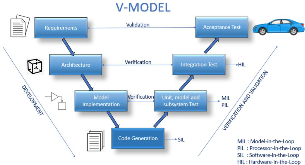
**Figure 3.1:** General V-Model diagram. Note: Taken from Model-Based Design (MBD) approach, by Jadhav[13].
