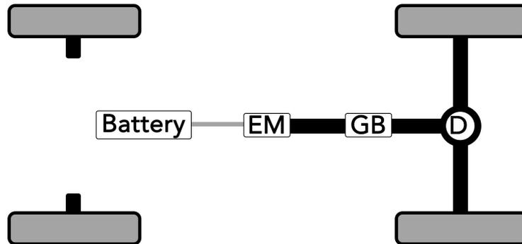
**Figure 2.13:** Powertrain architecture used in the HD Truck. Note: Adapted from the 2015 study, *Powertrain architectures of electrified vehicles: Review, classification, and comparison* [4].
