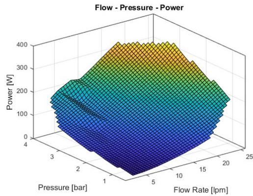
**Figure 5.16:** Power as a function of Flow Rate and Pressure.
