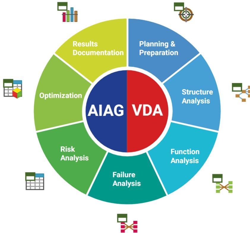
**Figure 4.7:** AIAG VDA 7-Step FMEA. Note: Taken from: *AIAG VDA 7 Step FMEA. Planning & preparation. Results documentation* [21].
