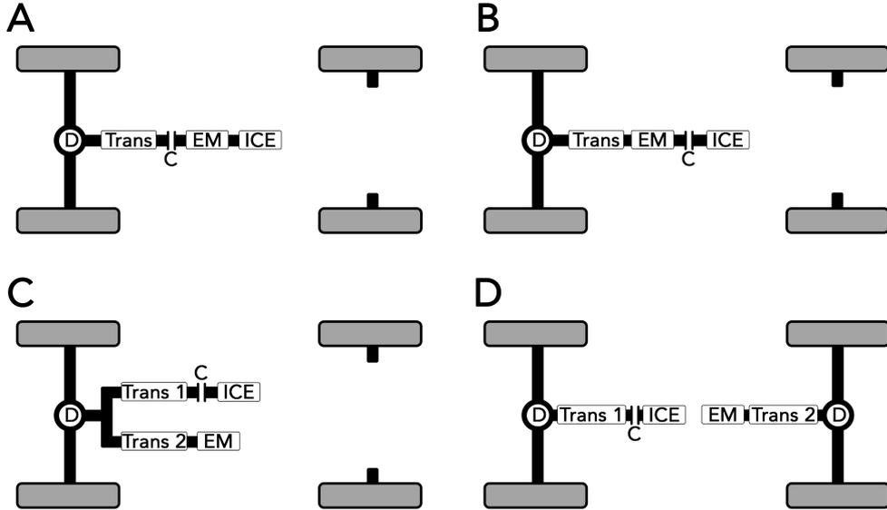
**Figure 2.3:** Some of the most common architectures for parallel HEVs. Note: Adapted from the 2015 study, *Powertrain architectures of electrified vehicles: Review, classification, and comparison* [4].
