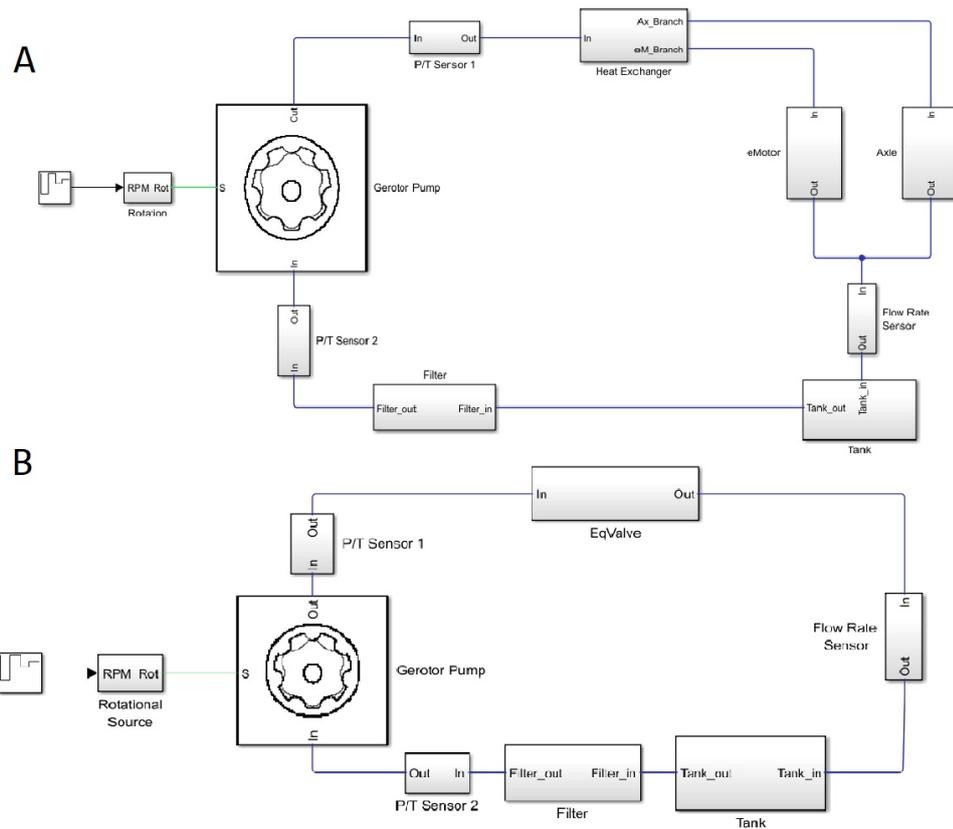
**Figure 5.13:** Generation of the EqValve Block Based on Individual Components.
