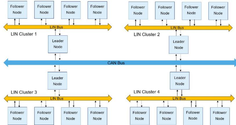
**Figure 6.5:** LIN in a Vehicle Note: Taken from *Local Interconnect Network (LIN)*, 2023 [27].
