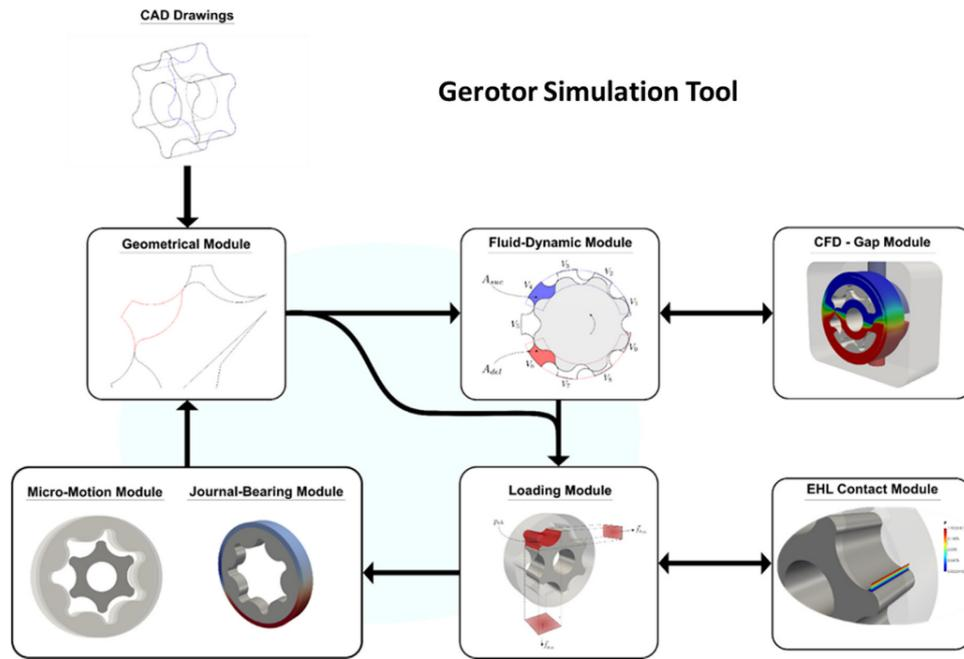
**Figure 5.1:** Different Model Types and Stages for a Gerotor Modelling and Simulation. Note: Adapted from 2020 paper, *A simulation model of Gerotor pumps considering fluid-structure interaction effects: Formulation and validation*, by Pellegrini et al. [9].
