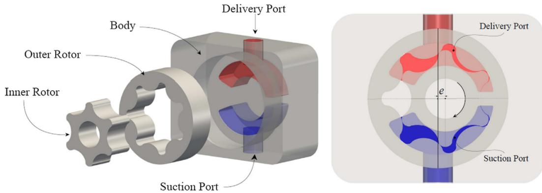
**Figure 2.8:** Construction of a typical Gerotor unit. Note: Adapted from 2020 paper, *A simulation model of Gerotor pumps considering fluid-structure interaction effects: Formulation and validation.* by Pellegrini et al. [9].
