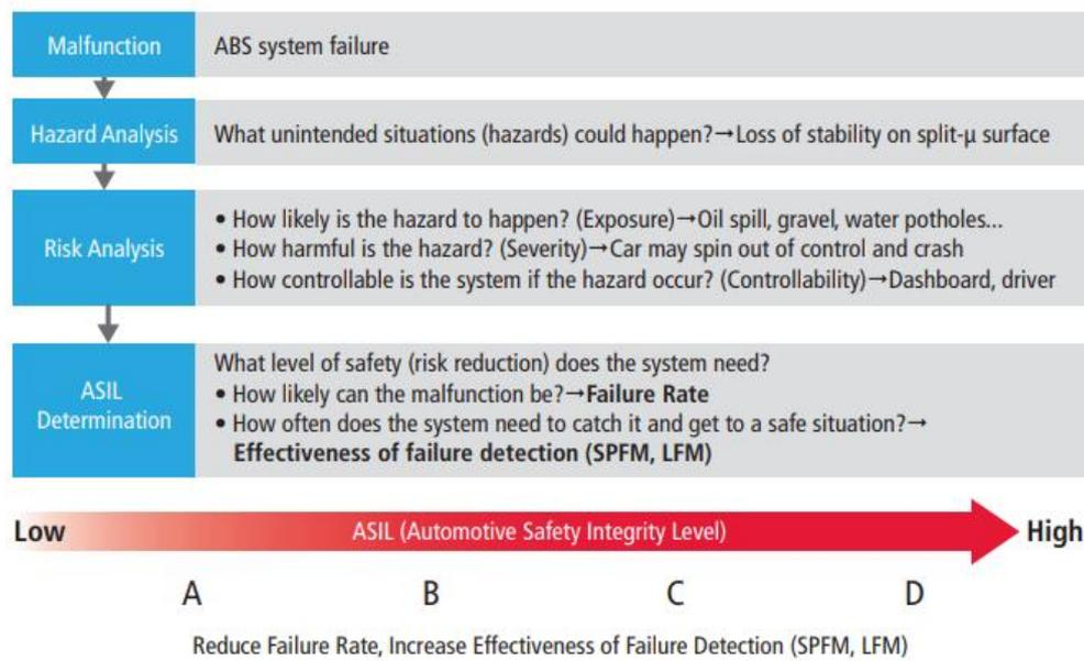
**Figure 4.1:** steps involved in the determination of ASIL for an Anti-Breaking System ( ABS). Note: Taken from *Through the Lens of ISO 26262 Paradigm: What is Functional Safety and ASIL* [15].
