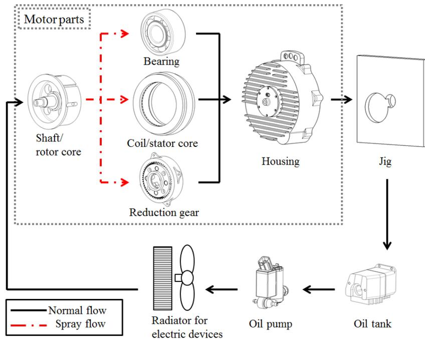
**Figure 2.7:** Flow circuit of the spray cooling system. Note: Adapted from the 2014 paper, *Performance Evaluation of an In-Wheel Motor Cooling System in an Electric Vehicle/Hybrid Electric Vehicle* by Lim et al. [8]
