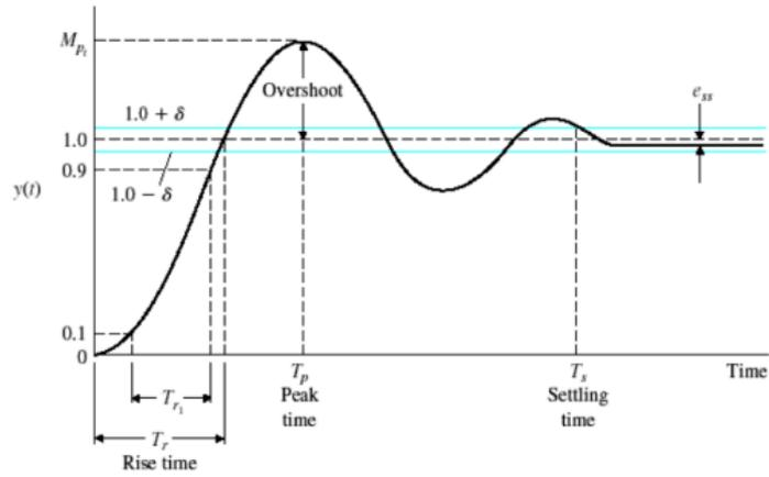
**Figure 2.17:** Step Response Parameters. Note: Taken from 2013 paper, *Matlab/GUI based basic design principles of PID controller in AVR* by Bayram et al [12].
