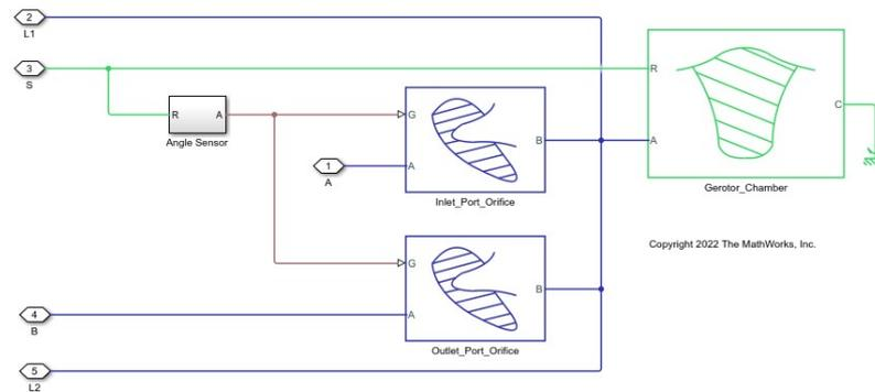
**Figure 5.5:** Modeling of the inner chambers and orifices according to the geometry parameters of the gerotor pump by MathWorks. Note: Adapted from *Gerotor Pump*. by MATLAB & Simulink - MathWorks Italia [22].
