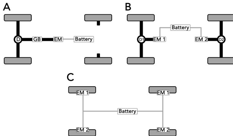
**Figure 2.1:** Some of the most common architectures for PEVs. Note: Adapted from the 2015 study, *Powertrain architectures of electrified vehicles: Review, classification, and comparison* [4].
