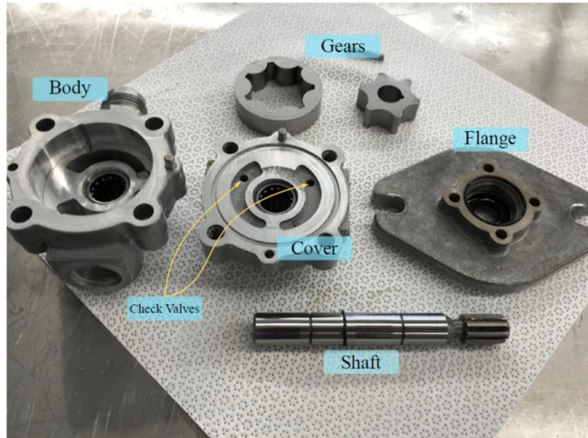
**Figure 5.6:** Physical gerotor pump decomposition performed by Pellegrini et al. Note: Adapted from 2020 paper, *A simulation model of Gerotor pumps considering fluid-structure interaction effects: Formulation and validation.* by Pellegrini et al. [9].
