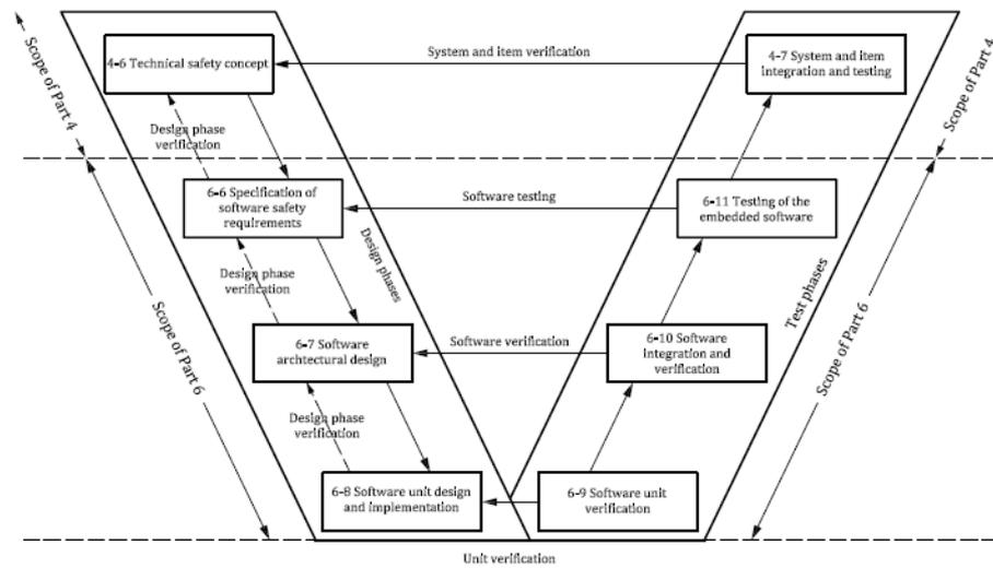
**Figure 4.5:** Reference Phase Model for the Software Development Note: Taken from *Freedom from interference FFI [19]*.
