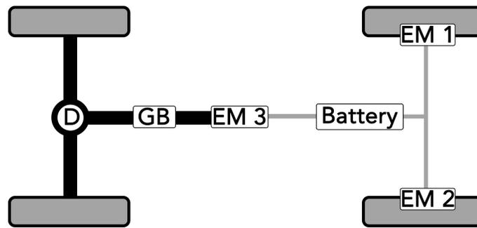
**Figure 2.9:** Powertrain architecture used in the Passenger Vehicle. Note: Adapted from the 2015 study, *Powertrain architectures of electrified vehicles: Review, classification, and comparison* [4].
