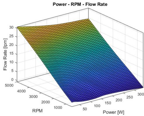
Figure 5.17: Flow Rate as a function of Power and RPM.
