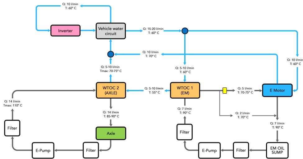
Figure 2.14: Hydraulic Circuit Layout No.1. as Proposed for The Client.
