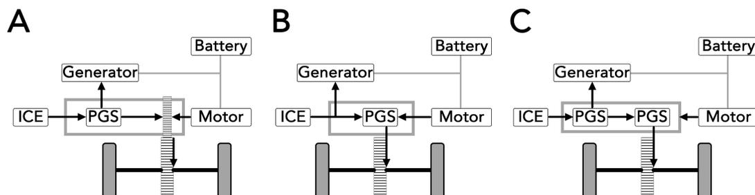
**Figure 2.4:** Some of the most common power-split architectures. Note: Adapted from the 2015 study, *Powertrain architectures of electrified vehicles: Review, classification, and comparison* [4].
