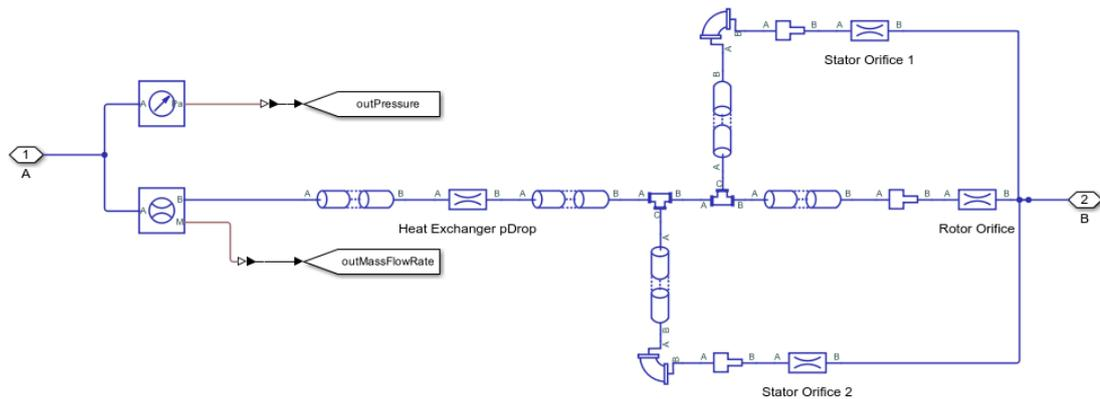
**Figure 5.12:** Modeling of the Load Components Conforming the Hydraulic Circuit by MathWorks. Note: Adapted from *Gerotor Pump*. by MATLAB & Simulink - MathWorks Italia.[22]
