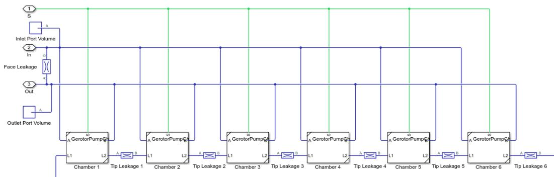
**Figure 5.3:** Modeling of the inner chambers and leakage of the gerotor pump by MathWorks. Note: Adapted from *Gerotor Pump*. by MATLAB & Simulink - MathWorks Italia [22].
