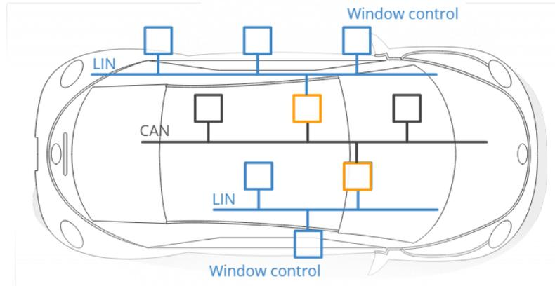
**Figure 6.3:** CAN and LIN as Communication Protocols in a Vehicle. Taken from 2021 Electronics [25].
