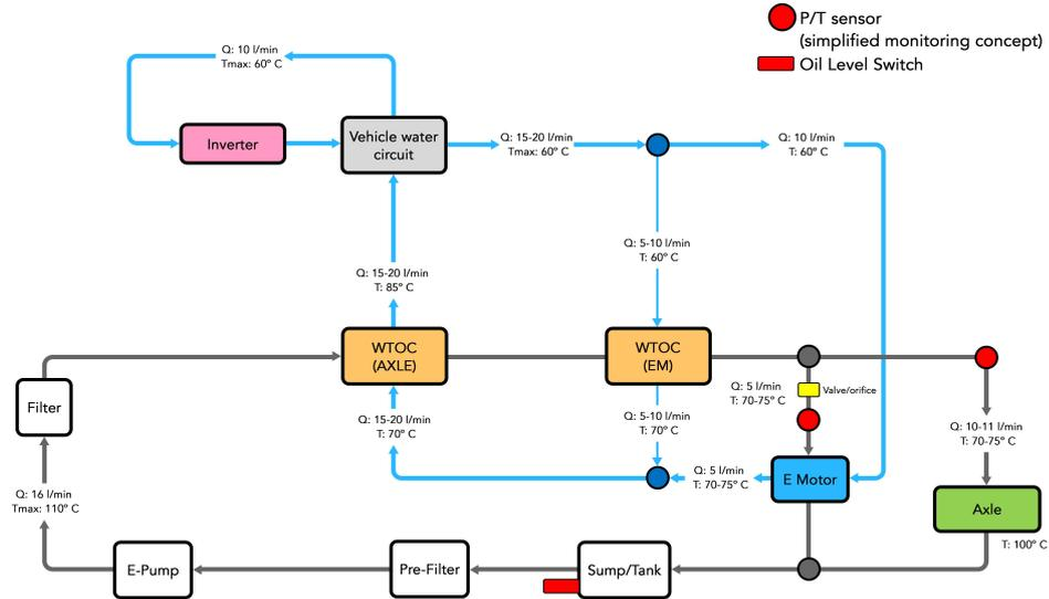
**Figure 2.15:** Hydraulic Circuit Layout No.2 as Proposed for The Client.
