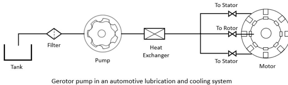
**Figure 5.2:** Scheme studied by MathWorks. Note: Adapted from *Gerotor Pump*, by MATLAB & Simulink - MathWorks Italia [22].
