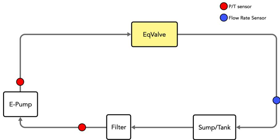
**Figure 4.10:** Integration of the Flow Rate sensor.
