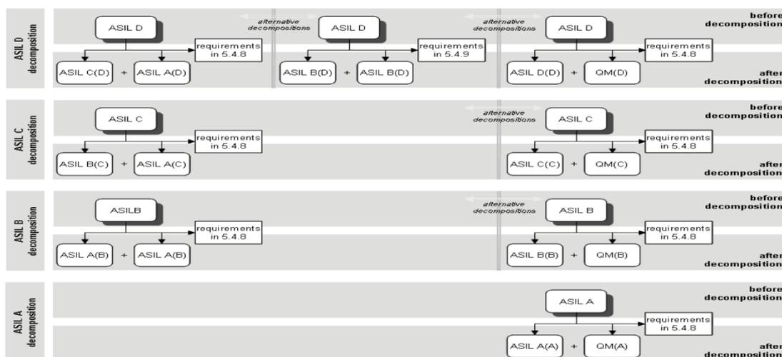
**Figure 4.6:** ASIL decomposition scheme. Note: Taken from *The Automotive Standard ISO 26262, the Innovative Driver for Enhanced Safety Assessment & Technology for Motor Cars* [20].
