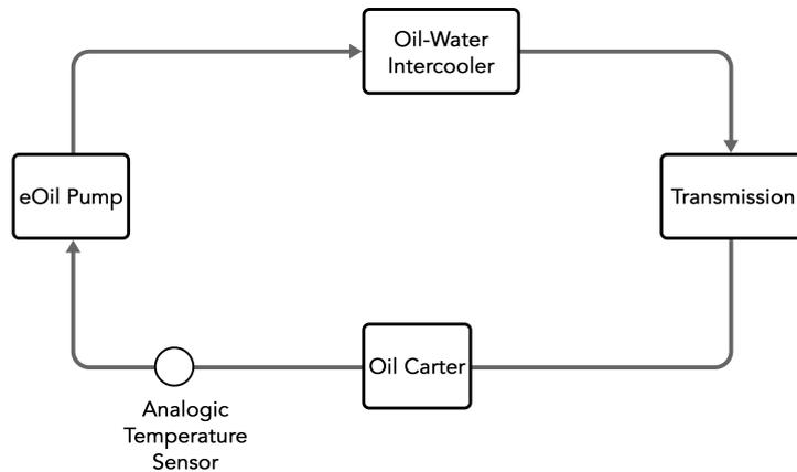
**Figure 2.11:** Representation of the Hydraulic Circuit Layout as Proposed by The Client.
