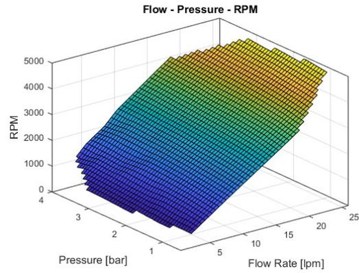
**Figure 5.15:** RPM as a function of Flow Rate and Pressure.
