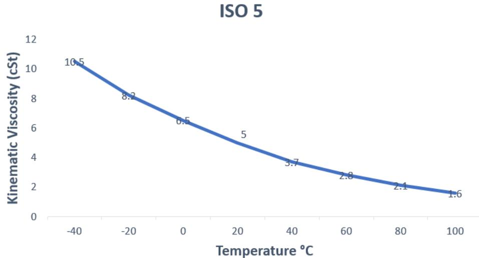
**Figure 3.8:** Test-Oil Characteristic Curve Generated Based on Information Provided by Suppliers.
