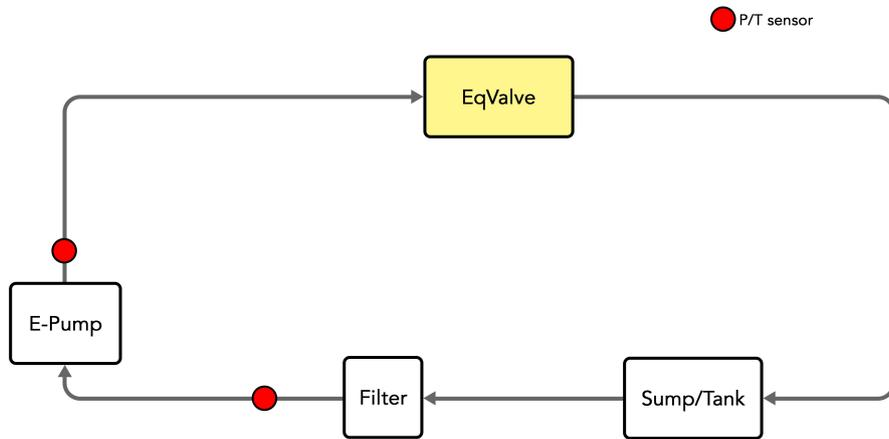
**Figure 4.9:** Double P/T sensor.
