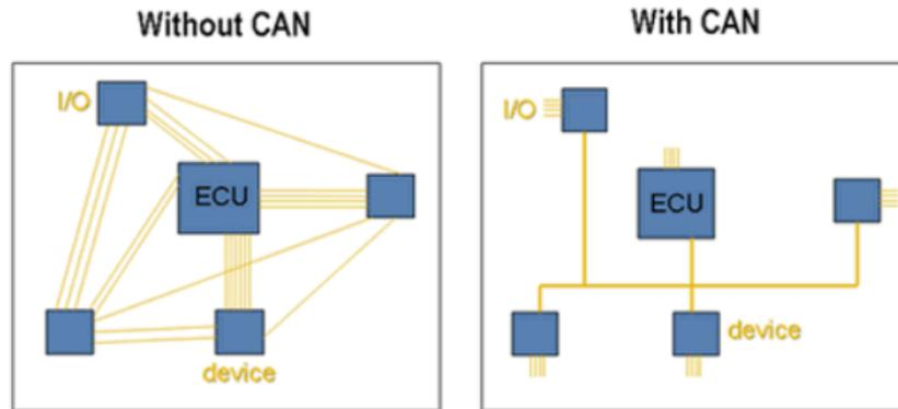
**Figure 6.4:** Effect of CAN on Automotive Application Note: Taken from: *CAN Bus Protocol - 10 Minute Lesson* [26].
