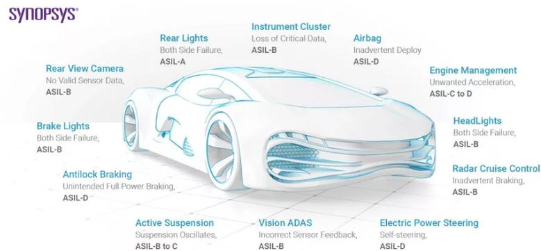
**Figure 4.2:** Some typical types of ASIL. Note: Taken from *What is ASIL (Automotive Safety Integrity Level)? – Overview: Synopsys Automotive* [16].
