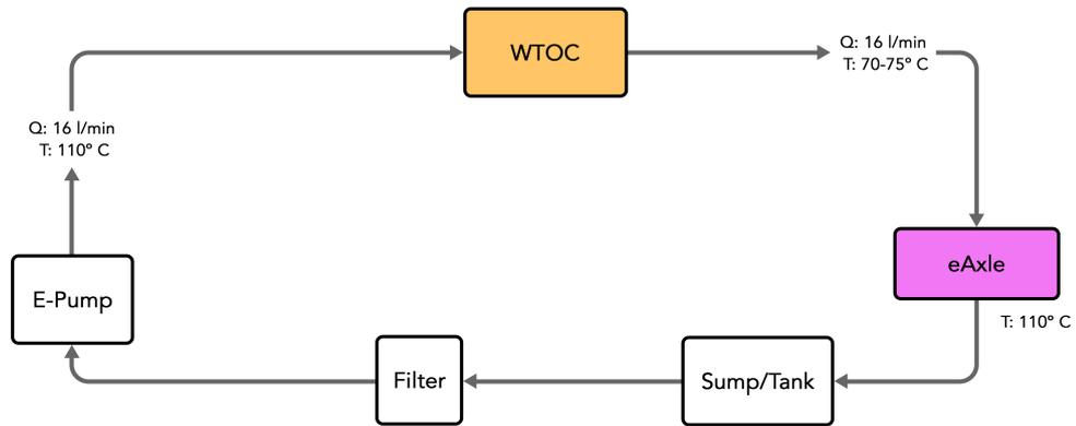
**Figure 3.6:** Final Placement of the Oil Filter.
