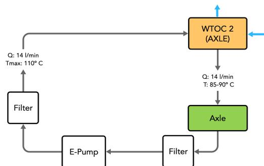
**Figure 3.4:** Isolation of the Axle Inner Loop in Layout No.1.
