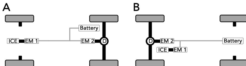
**Figure 2.2:** Some of the most common architectures for series HEVs. Note: Adapted from the 2015 study, *Powertrain architectures of electrified vehicles: Review, classification, and comparison* [4].
