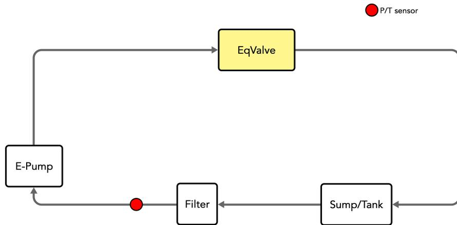
**Figure 4.8:** Initial placement of the P/T sensor.
