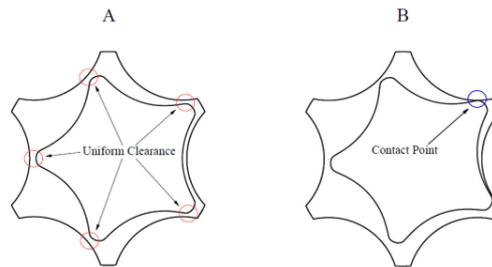
**Figure 5.4:** Difference between the presence of a uniform clearance (A) and a contact point (B). Note: Adapted from 2020 paper, *A simulation model of Gerotor pumps considering fluid-structure interaction effects: Formulation and validation* by Pellegri et al. [9].
