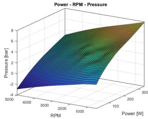
Figure 5.18: Pressure as a function of Power and RPM.
