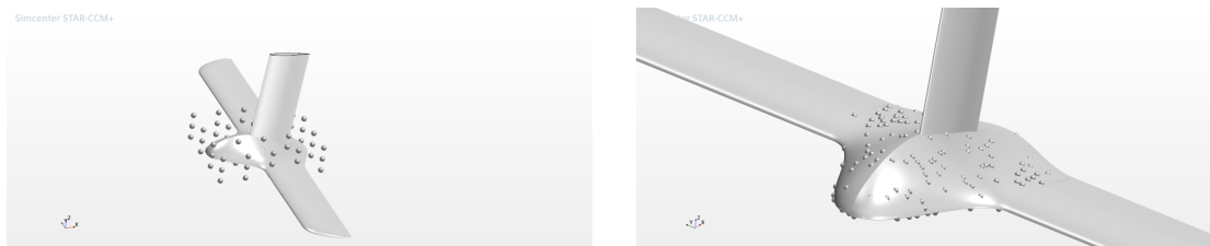
Figure 5.4: Two different control point configurations: box shape and directly on the bulb surface.
