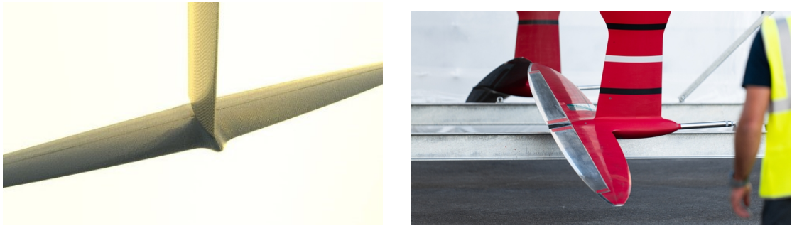
Figure 1.5: Two different joint configurations: a moth main foil (on left) and an Ineos T6's foil (on right).
