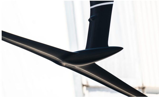
Figure 1.6: Detail of Luna Rossa LEQ12's right foil (2023).
