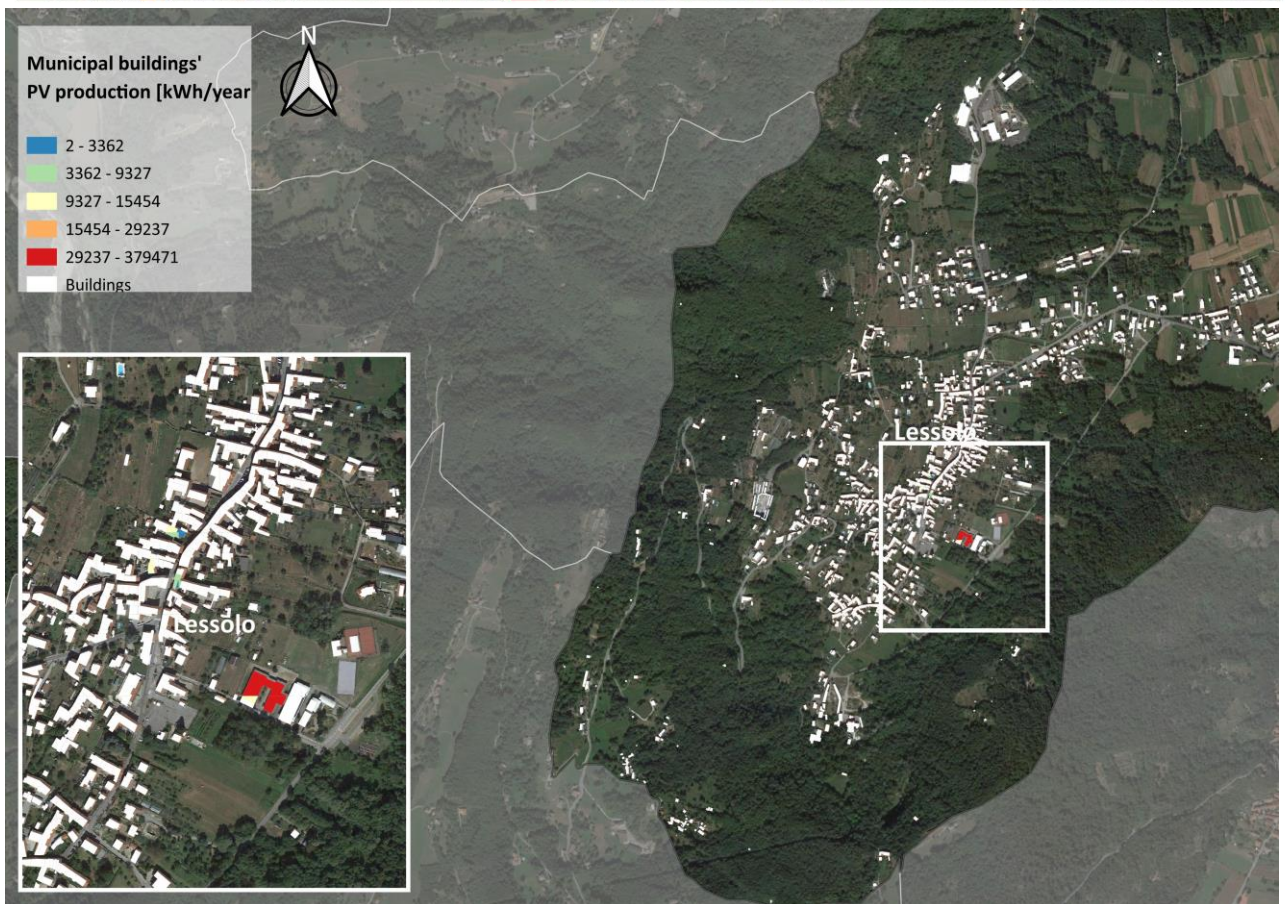
Figure 19: Lessolo global and Municipal buildings' PV production (personal elaboration)
