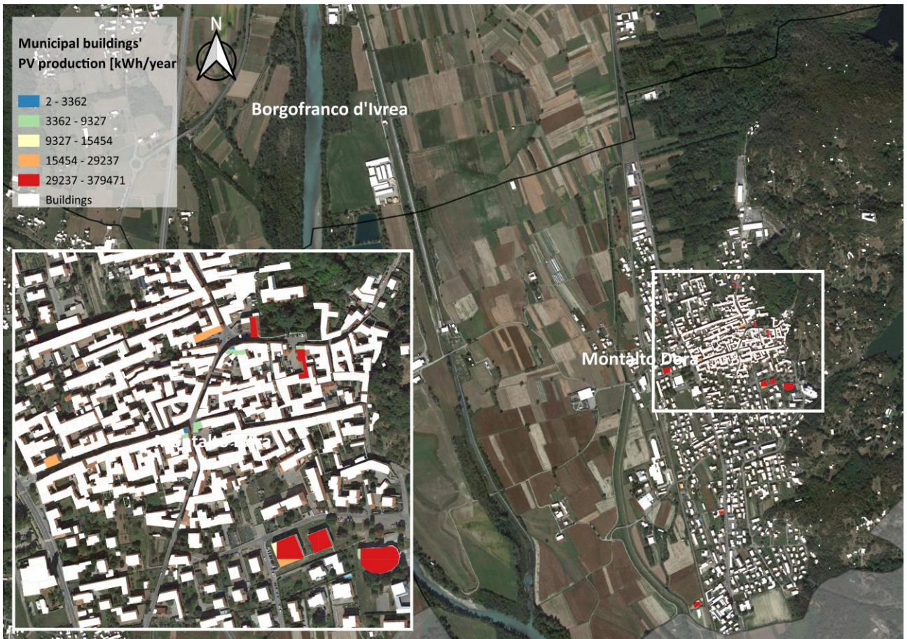
Figure 25: Montalto Dora global and Municipal buildings' PV production (personal elaboration)
