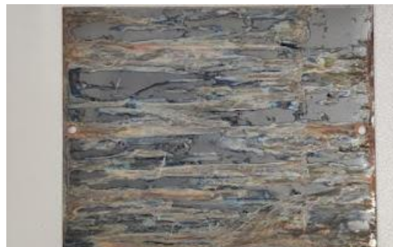
Figure 7.68 WC coating after 4 -5 days in the chamber.
