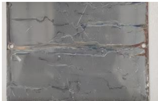
Figure 7.67 DLC coating after 4-5 days in the chamber.
