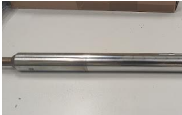
Figure 7.62 Hexavalent chrome before keeping in the chamber.
