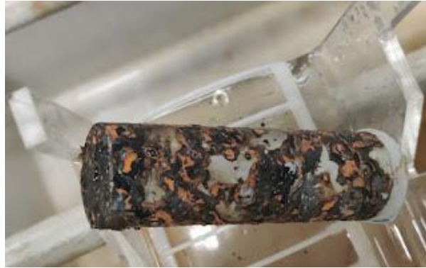
Figure 7.60 Fully corroded trivalent sample.
