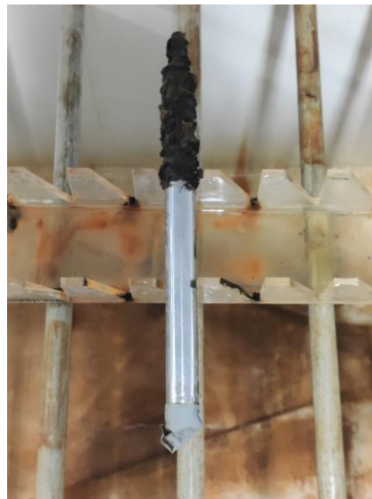
Figure 7.63 Hexavalent chromium after one month in corrosion chamber.
