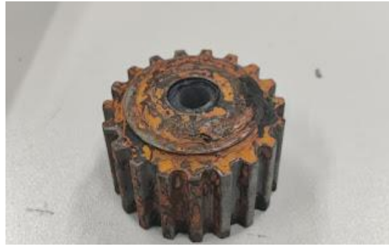
Figure 7.64 Sample E after 2 days in the chamber.
