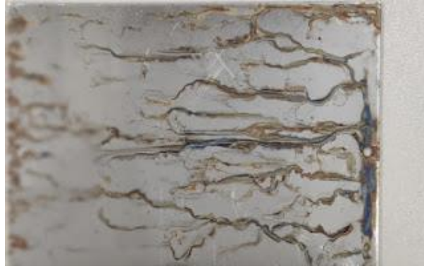
Figure 7.69 CrN coating after 4-5 days in the chamber.
