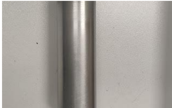
Figure 7.61 Trivalent sample before subjecting to corrosion.
