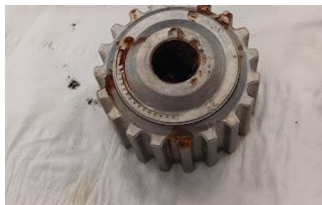
Figure 7.66 Sample D after one month in the corrosion chamber.
