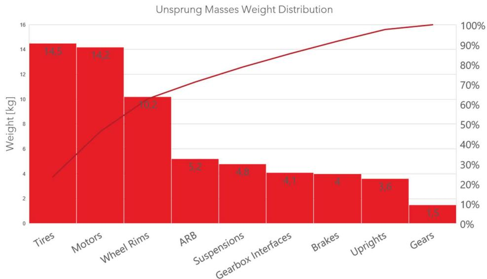
Figure 17. Pareto diagram of SC22 EVO unsprung masses
