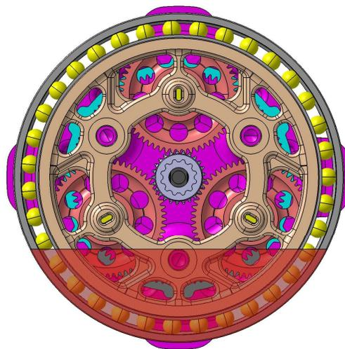
*Figure 104. Gearbox oil level*
