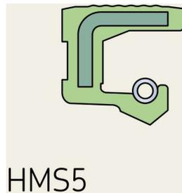
*Figure 107. HMS5 seal cross section*
