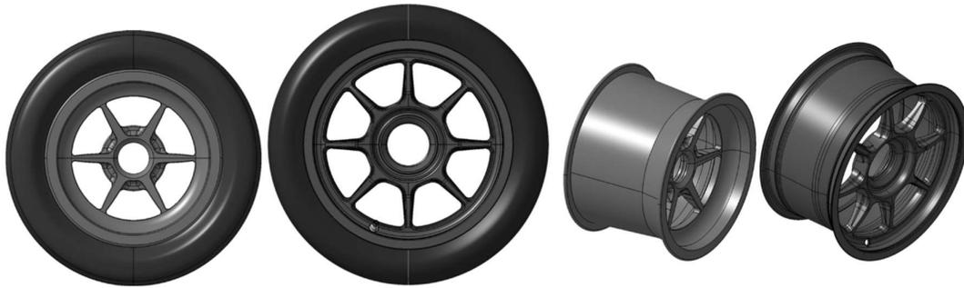
*Figure 18. 10" vs 13" wheels comparison*
