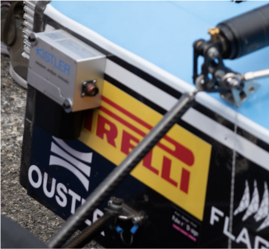
Figure 6.1: Kistler Ground Speed Sensor mounted on car
