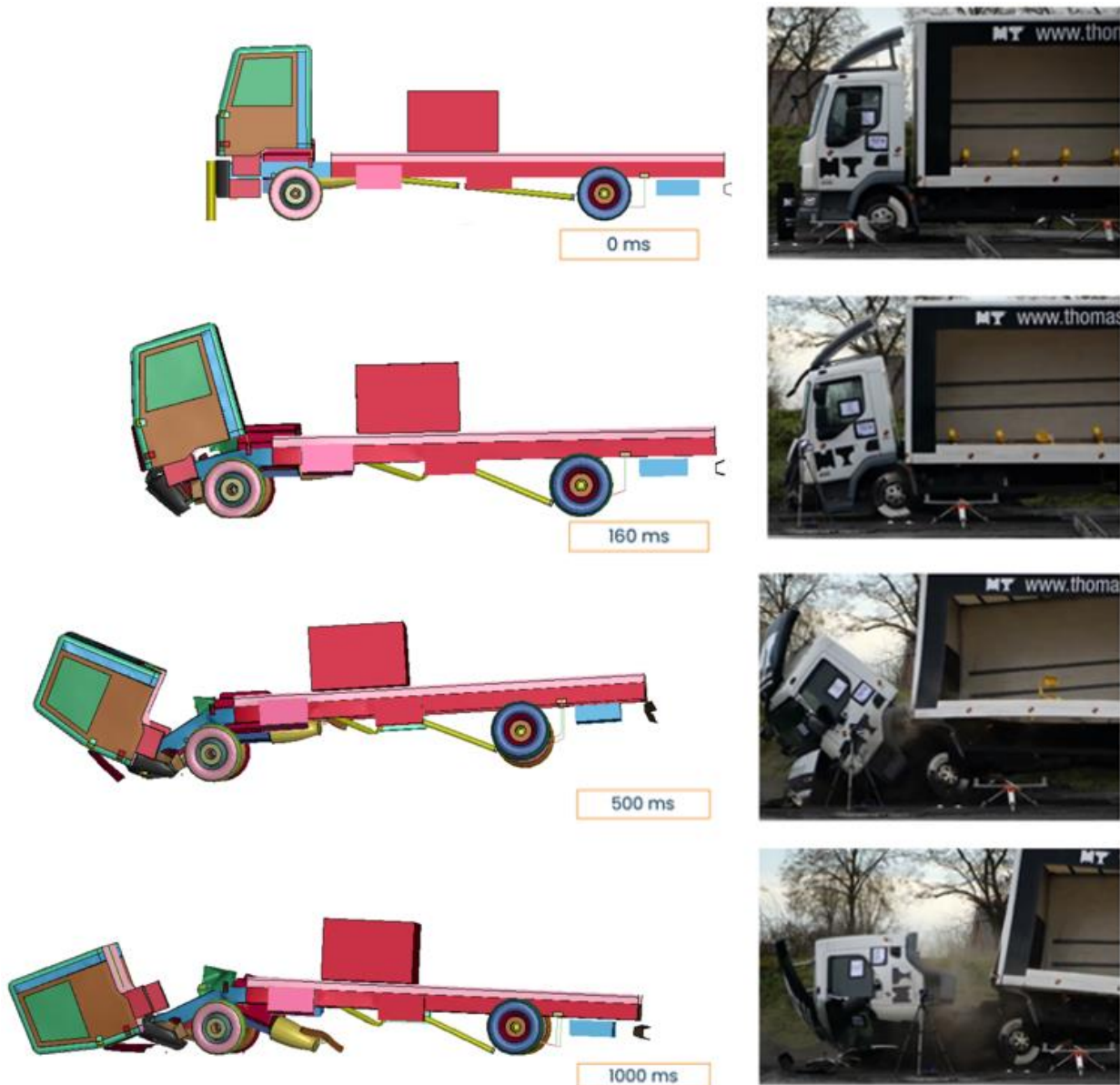
Figure 4.27 – Bollard at \frac{3}{4} engine animations comparison side view
