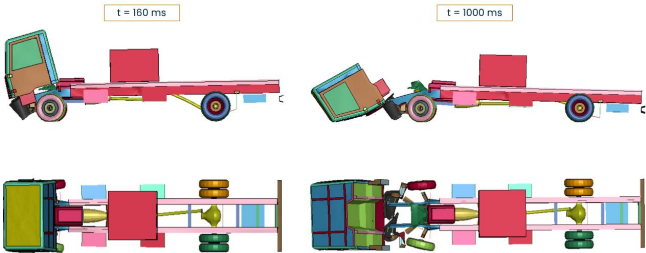
Figure 4.19 – Bollard offset: 0 mm – impact at 160 ms and 1000 ms
