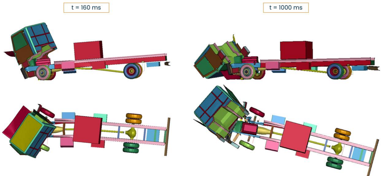
Figure 4.30 – Bollard offset: 400 mm – impact at 160 ms and 1000 ms
