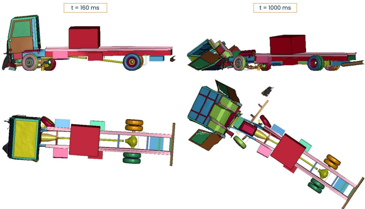
Figure 4.34 – Bollard offset: 750 mm – impact at 160 ms and 1000 ms
