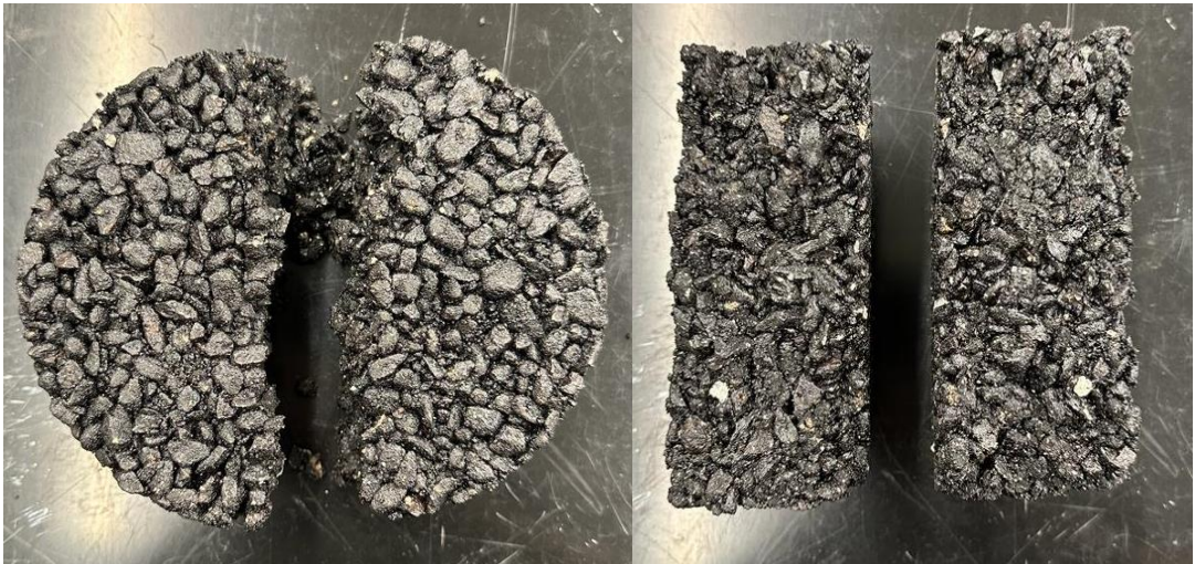
Figure 23. Failure surface of a specimen
