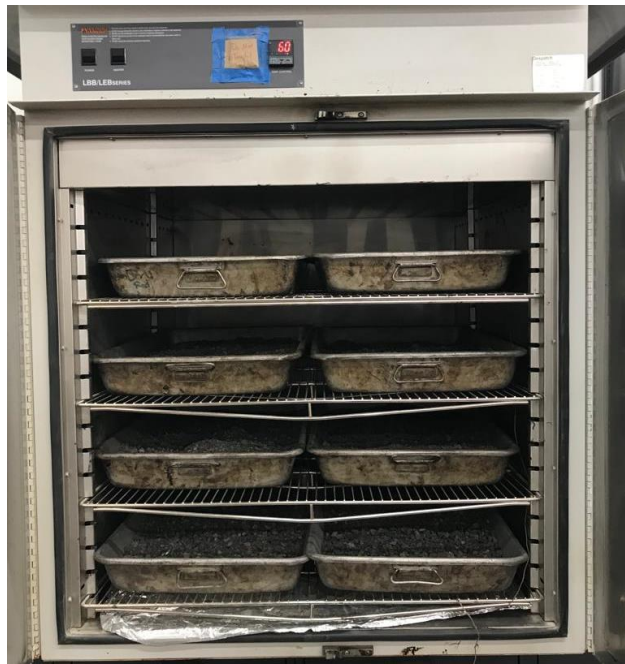
Figure 7. Aggregate/RAP drying oven
