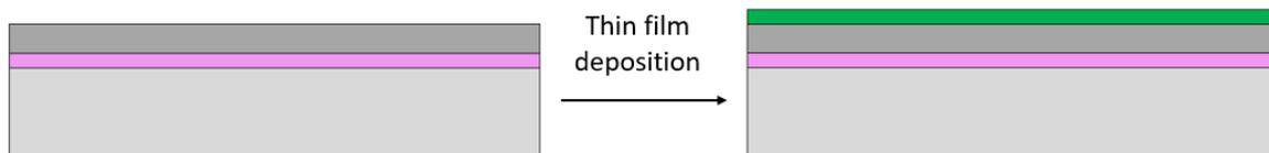
Figure 17: Scheme of the thin film deposition on an EPI Poly layer.
