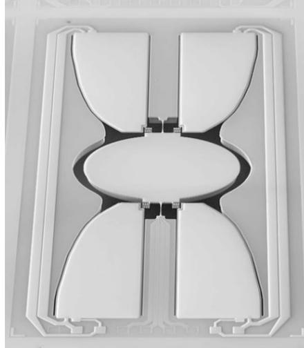
Figure 2: SEM image of a PZT-actuated micromirror. [2]
