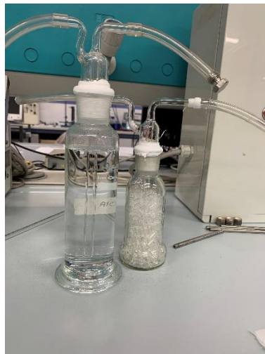
Immagine 4.3 on the left the Drexel of evaporation on the right the Drexel of condensation
