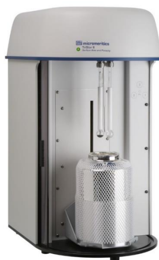
Figure 3.1 Physisorber of Nitrogen for physisorption Micromeritics TriStar II
