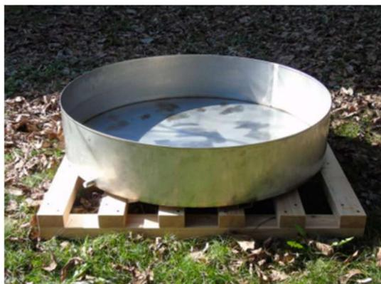
Figura 31: Evaporimetro di classe A (FONTE: GEOVES, *Monitoring Systems for environmental and renewable energy*)
