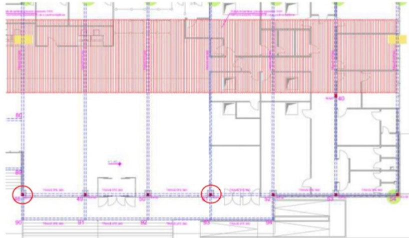
Figure 2.9: Discrepancies between record layouts and inspection survey. Column 51 and 48 in the records
