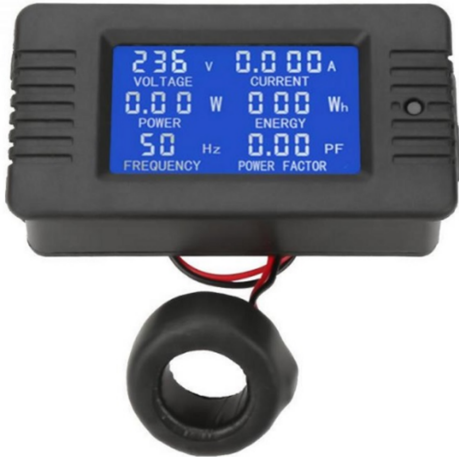
Figure 5.2: Device Used to Measure Server Energy
