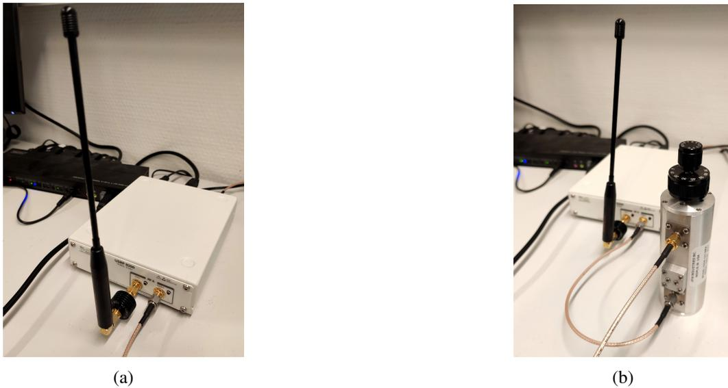
Fig. 5.6 URSP Radio (a) and Attenuator (b).
