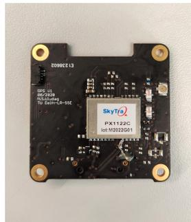
Fig. 5.3 SkyTraq PX1122C GNSS Receiver.
