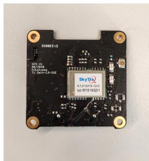
Fig. 5.4 SkyTraq S1216F8-GI3 GNSS Receiver.
