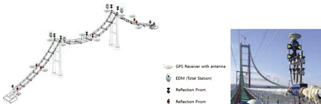
Figure 3-26: Survey equipment's arrangement for absolute sag [73]
