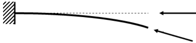
Figure 2-4: Follower force representative of wind action [5]
