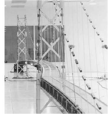
Figure 2-1: Akashi Kaikyo's deck deformations induced by wind [84]
