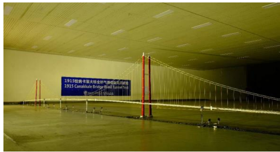
Figure 5-3: Deck sectional model (scale ratio at 1:130) (left); Full-bridge model (scale ratio at 1:190) (right) [78]
