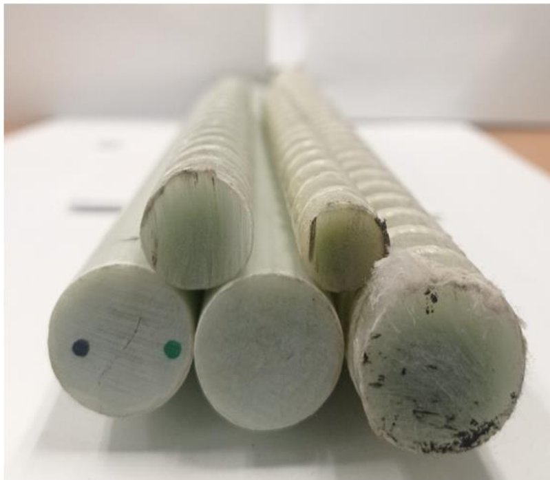
Figure 33: GFRP bars overall view
