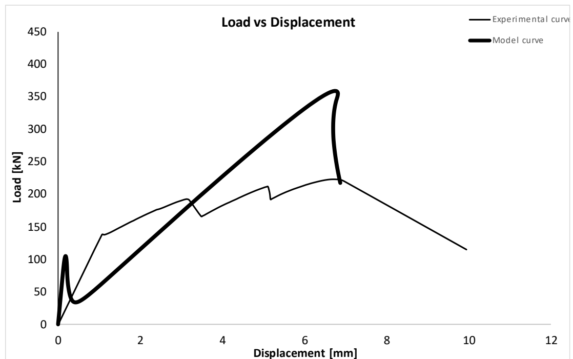
Graph 40: crushing point identification.
