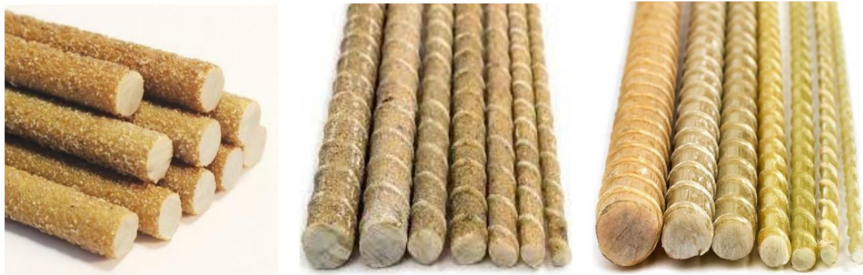
Figure 4: Sand coated, sand-helical wrapping, helical wrapping
