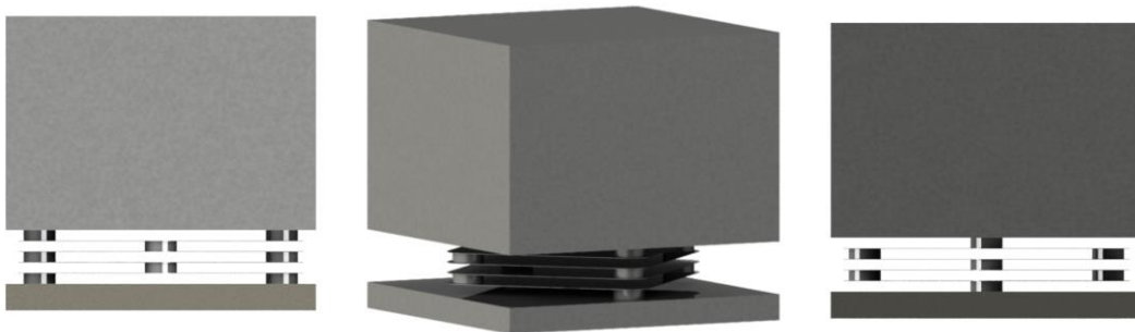
Fig. 4.3: Multiple sheets elastic suspension concept, front and side rendering view
