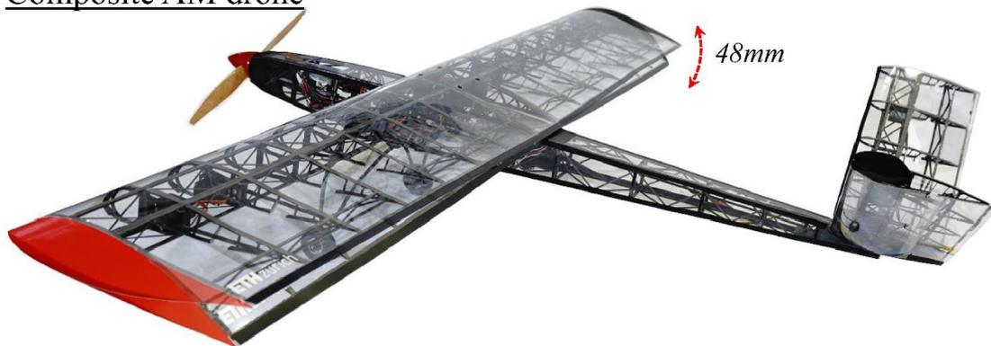
Figure 1.5: 3D printing manufactured composite morphing wing [10]
