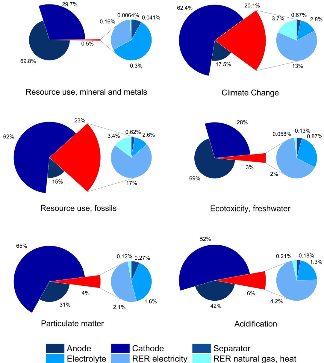
**Figure 4.2:** Contributions of each cell component and energy vector to the impacts of each battery cell.
