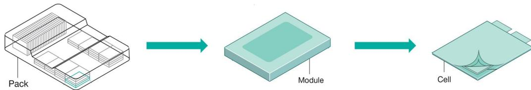
**Figure 2.12:** Disassembly Procedure of the Battery Pack
