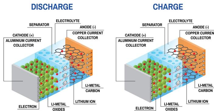
**Figure 2.1:** Lithium Ion Battery Cell in Charge (right) and Discharge (left) Phase [13]
