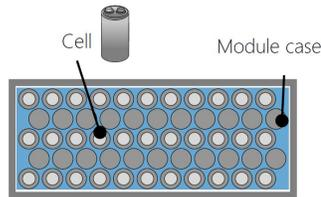
**Figure 2.5:** Cylindrical Cell Module [36]
