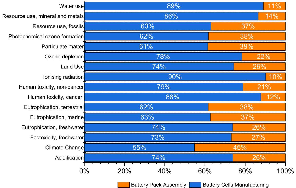
**Figure 4.1:** Contributions of cells manufacturing and pack assembly to the impacts of the battery pack.
