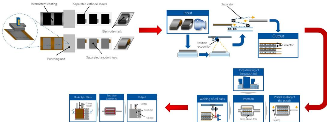
**Figure 2.2:** Assembly Procedure of Pouch Cell [35]
