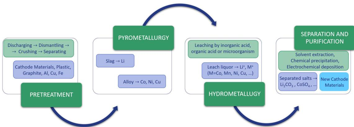
**Figure 2.13:** Overview of Pyro-Hydrometallurgical Recycling Process for LIBs
