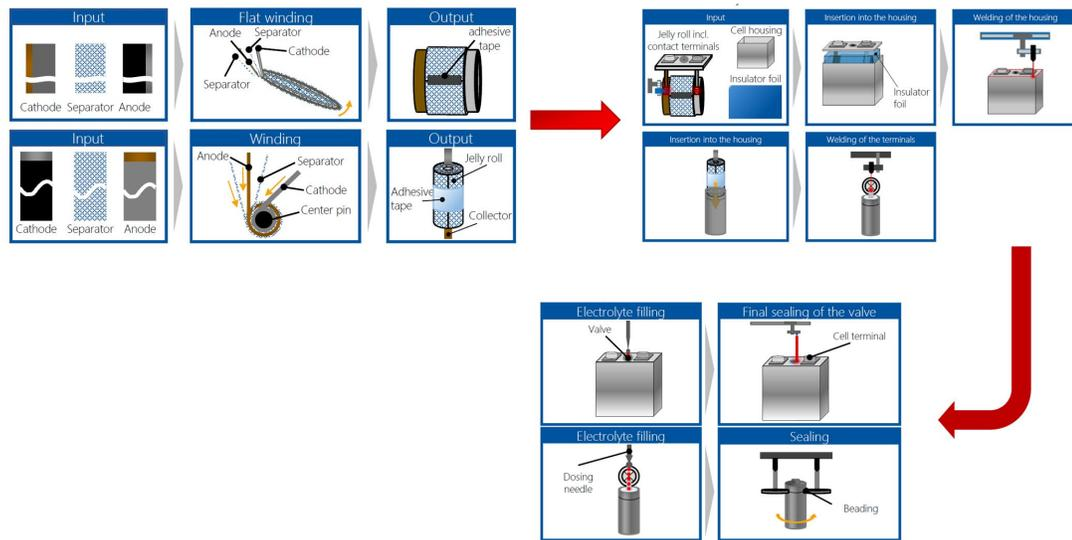
**Figure 2.3:** Assembly Procedure of Prismatic and Cylindrical Cell [35]
