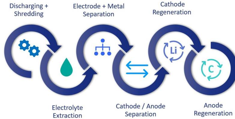
Figure 2.14: Overview of Direct Recycling Process for LIBs
