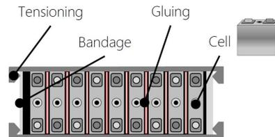
**Figure 2.6:** Prismatic Cell Module [36]
