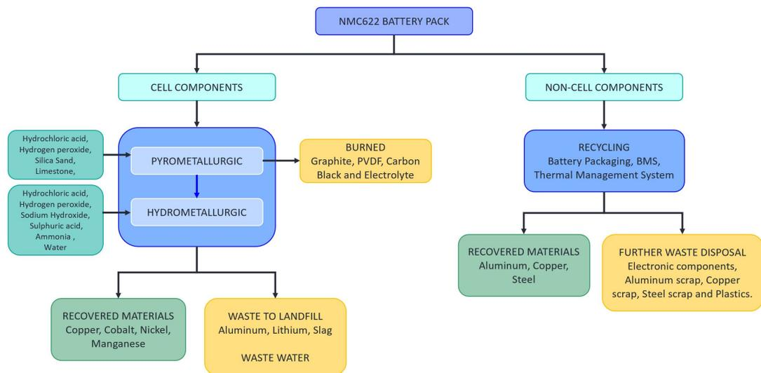
**Figure 3.1:** Pyro-Hydrometallurgic Process Implemented
