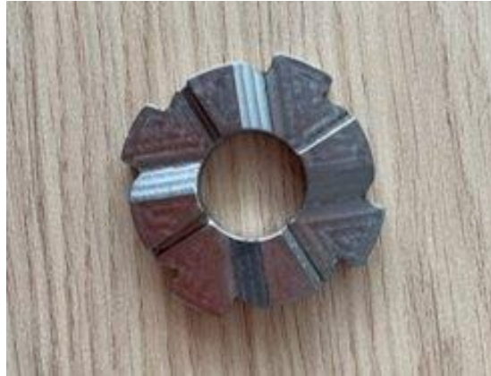
Figure 71: Electro-magnetic clutch's auxiliary disk
