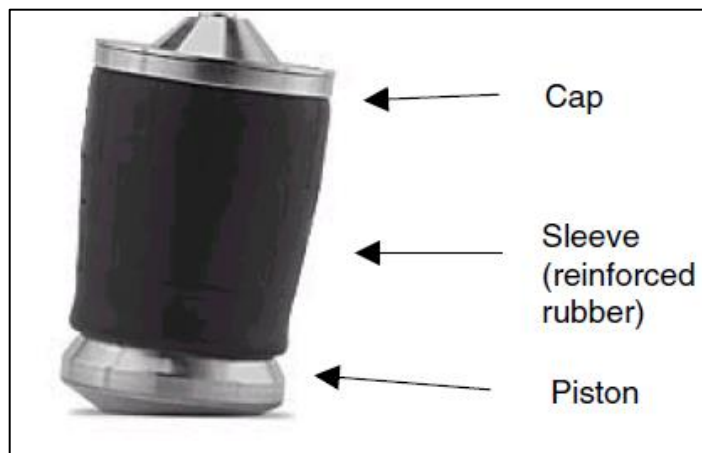
Figure 17: Rolling lobe air spring [11]
