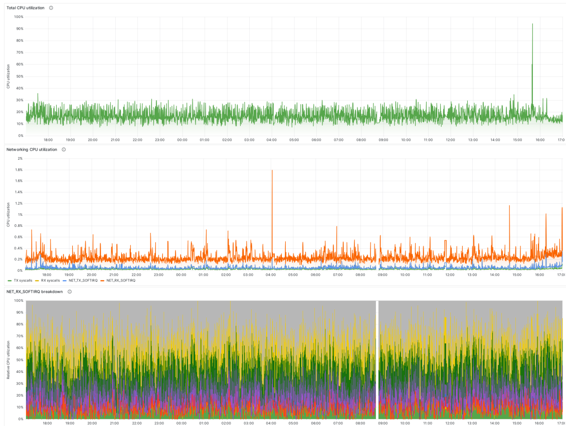
Figure 6.9: CPU utilization statistics of the CrownLabs worker4 node over a one-day observation period as captured by Netto and displayed by Grafana. The graphs show: overall CPU utilization (top), networking CPU utilization (middle) and breakdown of the NET_RX_SOFTIRQ (bottom).
