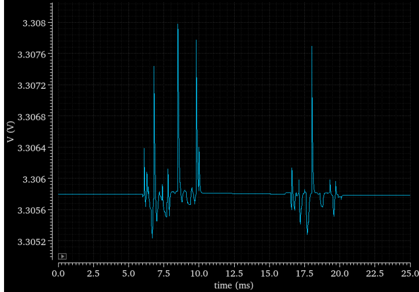
Figure 12: Example of a SEE simulation. This specific example considers the REG12V regulator and the graph shows his V_{out} . Every node in the circuit is tested with the proper current direction.
