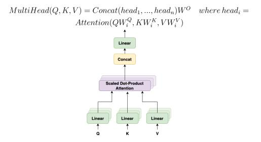
The Transformer uses multi-head attention in three different ways:
