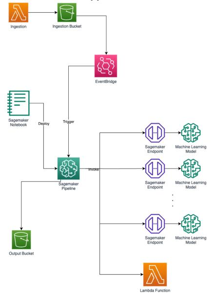
After the execution of the pipeline the results are stored into the Output S3 Bucket.
