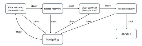
Figure 6.6: Schematic representation of the move base working conditions as a state machine.
