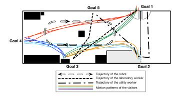
Figure 4.6: Ideal trajectories of the robot and the various types of pedestrians
