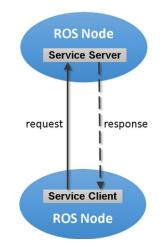
Figure 6.3: A schematic representation of the request/response communication paradigm implemented in ROS.
