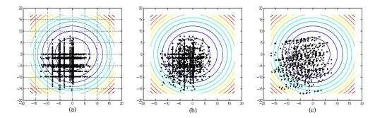
Figure 4.3: Effect of different values of Cr on a distribution of candidate trial vectors obtained by running DE on a single starting population of ten vectors for 200 generations with selection disabled [45]: (a) Cr = 0; (b) Cr = 0.5; (c) Cr = 1.
