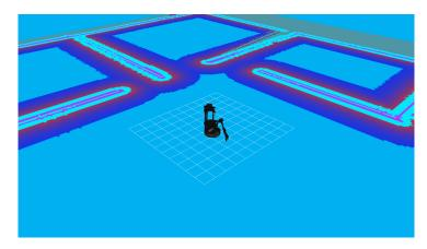
Figure 7.2: Example of locobot visualization in Rviz with the global costmap related to the obstacles (walls) in the environment.
