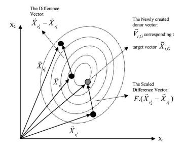
Figure 4.2: Standard DE-mutation in a 2-D parametric space
