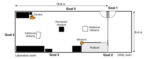
Figure 4.4: Schematic presentation of the laboratory room where the trajectories were recorded.
