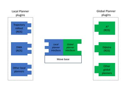
Figure 6.7: Schematic representation of move base local and global planner interfaces and plugins.
