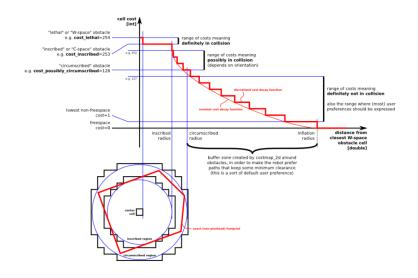
Figure 6.5: Costmap inflation process [94]. The value associated with the occupied cell is the maximum cost (254). This value decreases with increasing distance from the center of the obstacle. Lower cost represents a lower probability of collision hazard.
