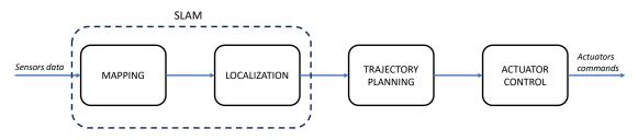
Figure 2.1: Main phases of autonomous navigation.
