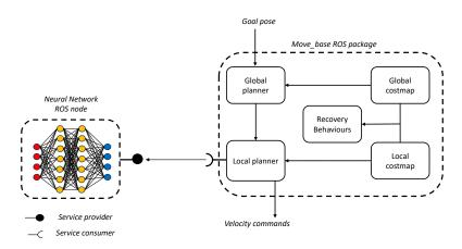
Figure 6.10: Representation of the final architecture implemented in ROS.
