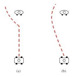
**Figure 2.4:** Comparison of trajectories generated by the two types of planner (from [12]): (a) Reactive: when a person appears in its way, the robot modify the local path to change direction; (b) Predictive planner: by exploting a human-motion model, the robot first predicts the future states of the person and then it computes its path considering the mutual avoidance.
