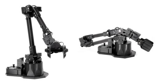
Figure 5.5: WidowX-250 6DOF Robot arm.
