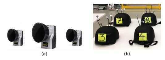
**Figure 4.5:** (a) Qualisys Oqus 7+ infrared cameras; (b) helmets with reflective markers, used to track pedestrians.
