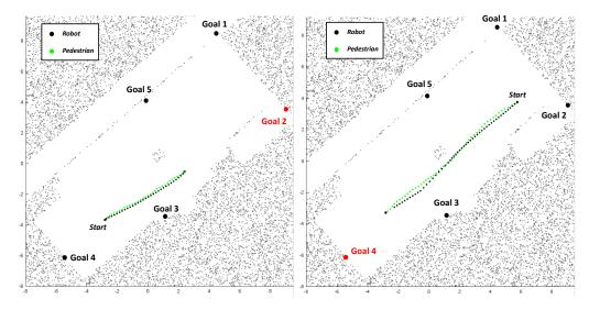
**Figure 4.8:** Comparison between real human trajectories contained in Thör (green) with the corresponding robot trajectories (black) obtained by using SFM parameters from DE estimation.
