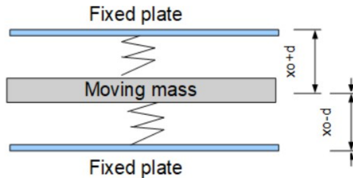
Figure 28: basic model of a capacitive accelerometer
