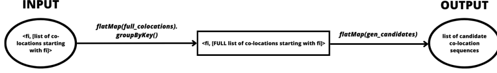
Figure 4.3. Architecture of the application to generate candidate co-location sequences
