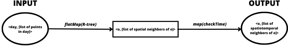
Figure 3.5. Structure of algorithm to compute spatio-temporal neighbors with R-tree
