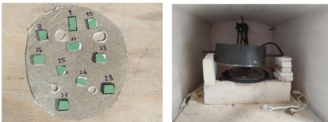
**Figure 2.5:** On the left there are all the samples prepared for the ageing test, with humid air (50%). On the right side, ageing test setup is shown.
