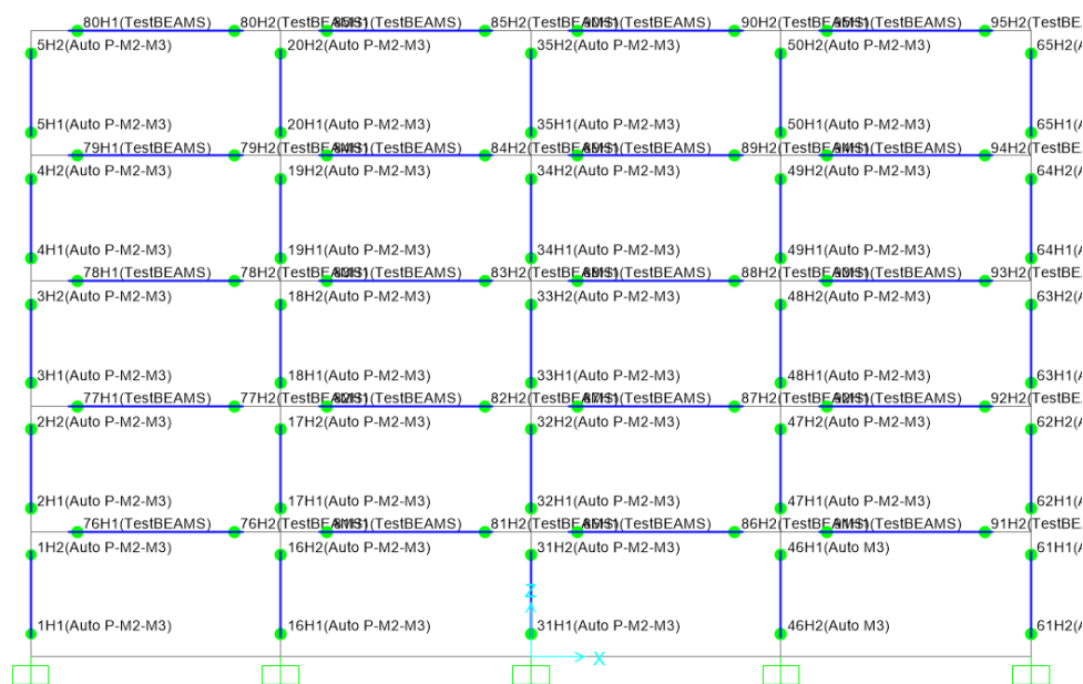
Figure 93 Position of the plastic hinges in the element in the existing structures, longitudinal frame.
