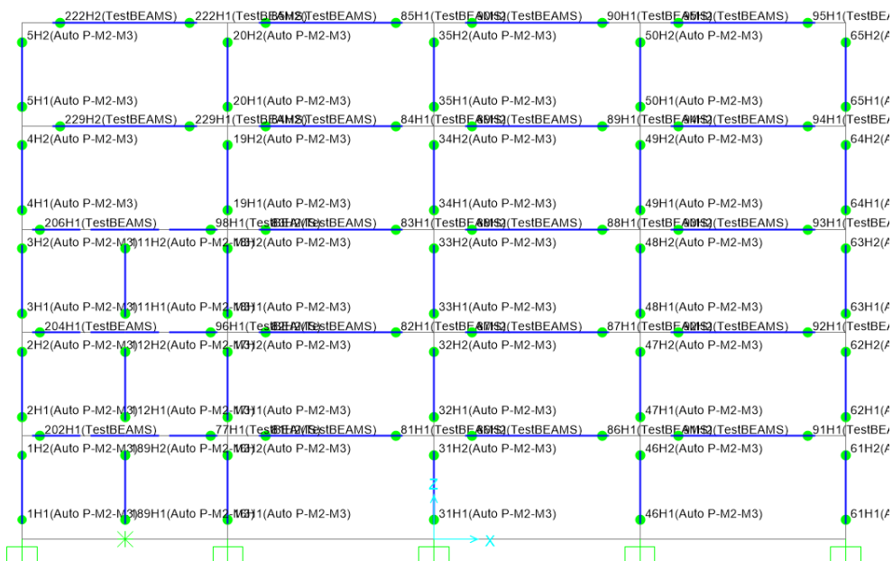
Figure 96 Position of the plastic hinges (green dots) in the elements of the reinforced concrete shear wall retrofit, case study in location 2, Aachen. Presence of one shear wall in a longitudinal frame.
