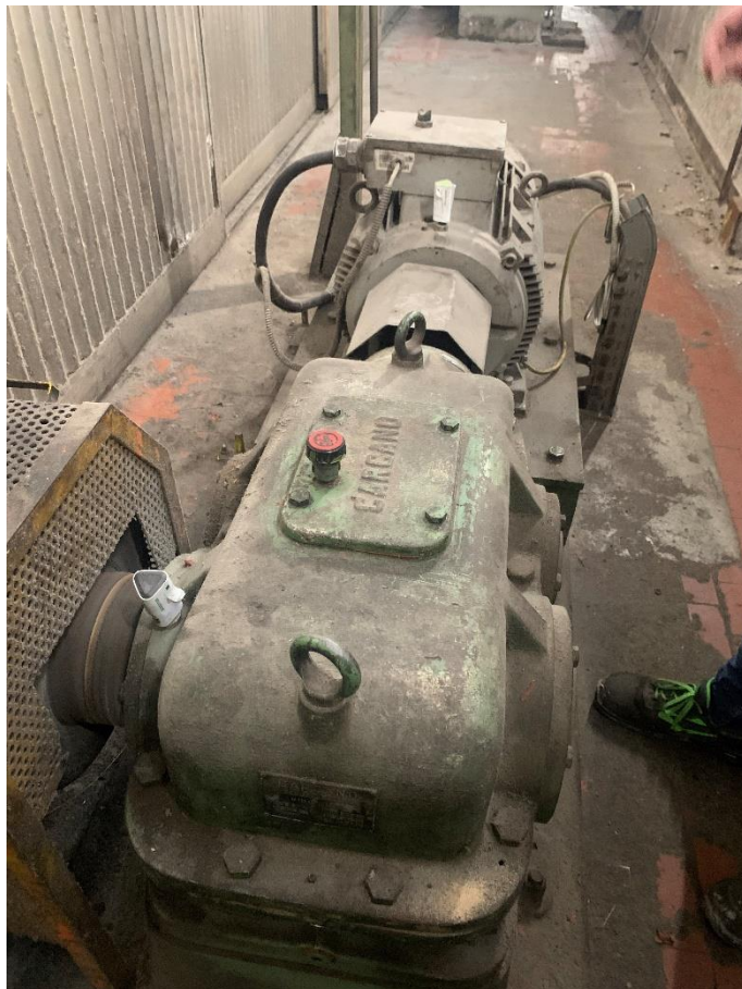
Figure 32: Motor-gearbox assembly with application of the sensors
