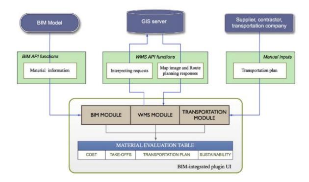
Figure 3.2.3.2 "Actors connected with BIM integratio"
