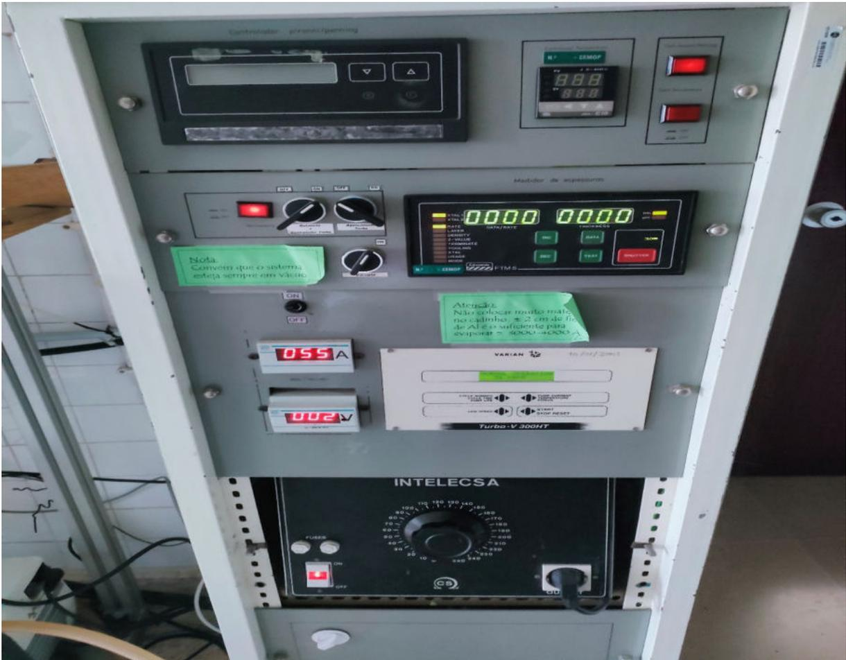
**Fig 2.3** The control panel of the thermal evaporator
