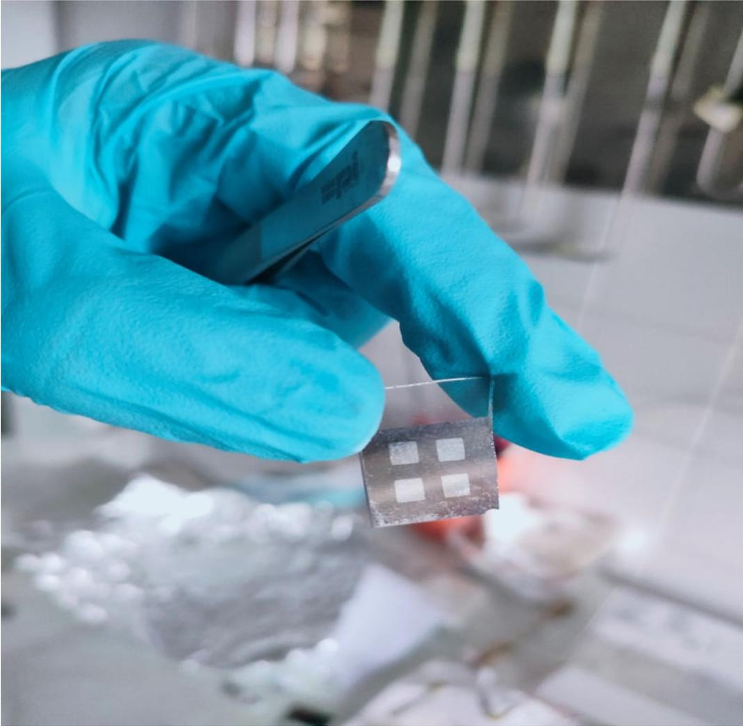
**Fig 3.1 Sample of three layers for Hall effect**
