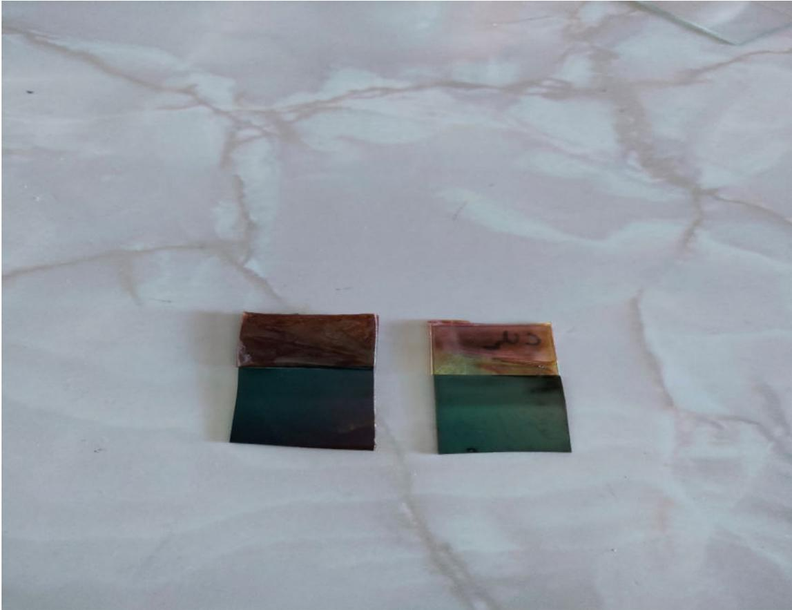
**Fig 3.19** a p-n junction made using CuO (on the left) and using Cu<sub>2</sub>O (on the right)
