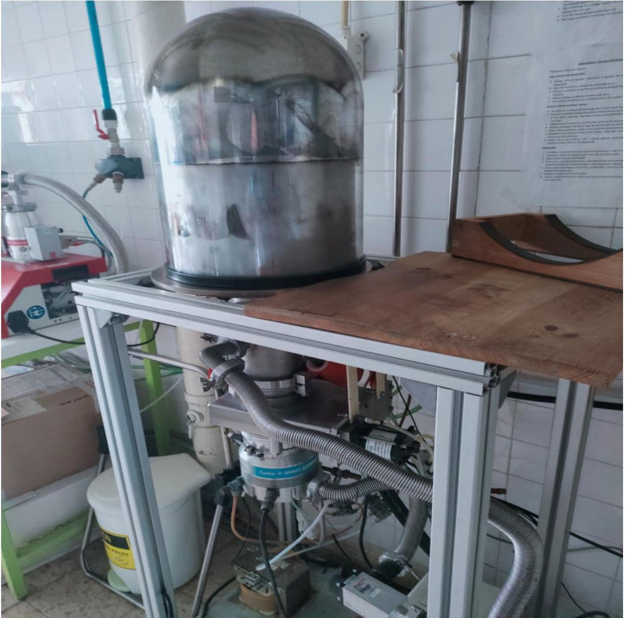
**Fig 2.4** The deposition chamber
