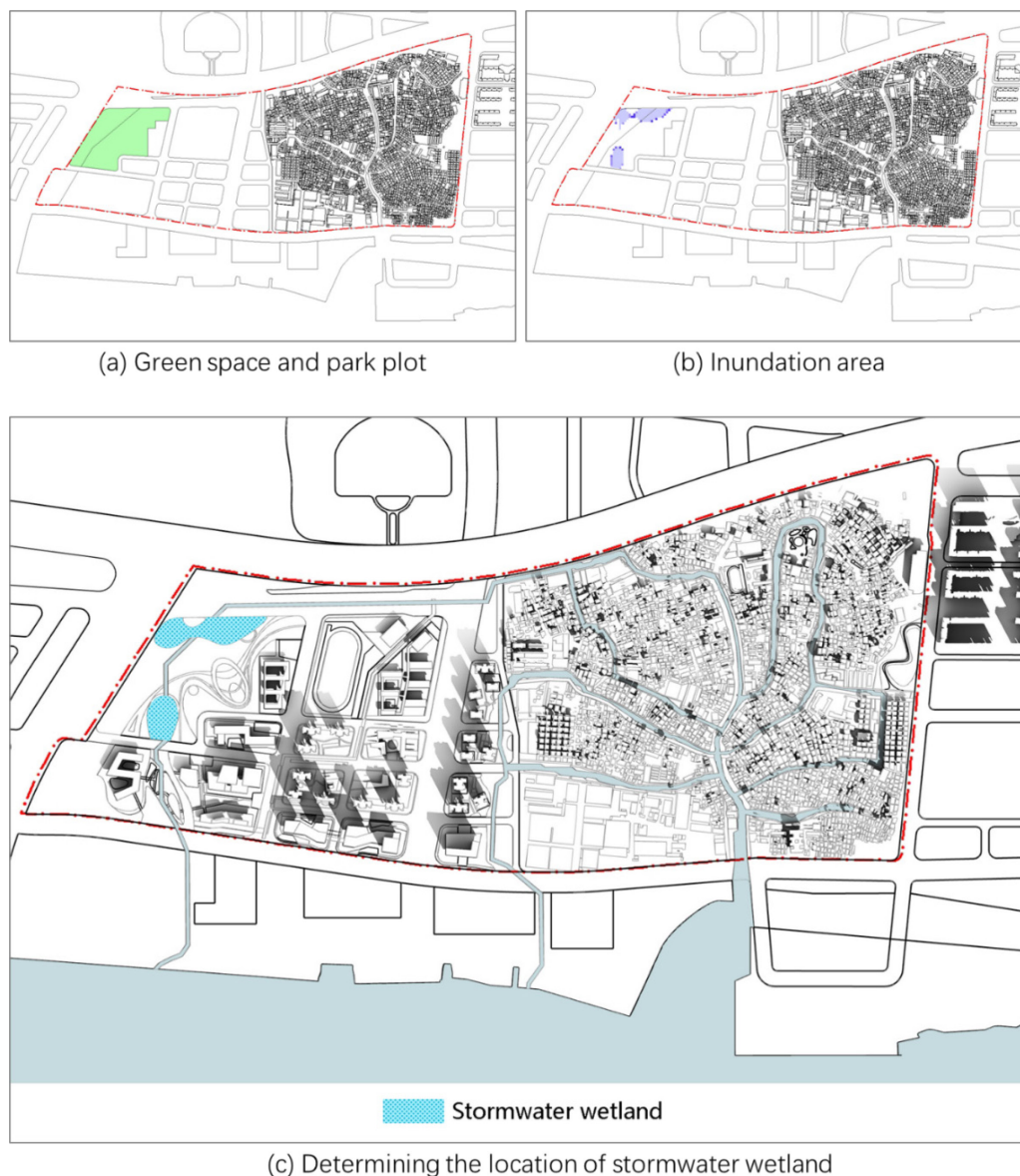
Figure 6-10 Layout process and results of the stormwater wetland
