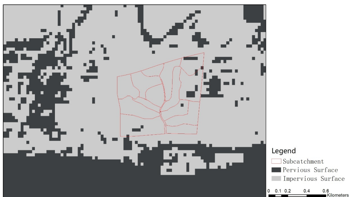
Figure 4-23 Impervious-surface distribution for the design horizon 2020
