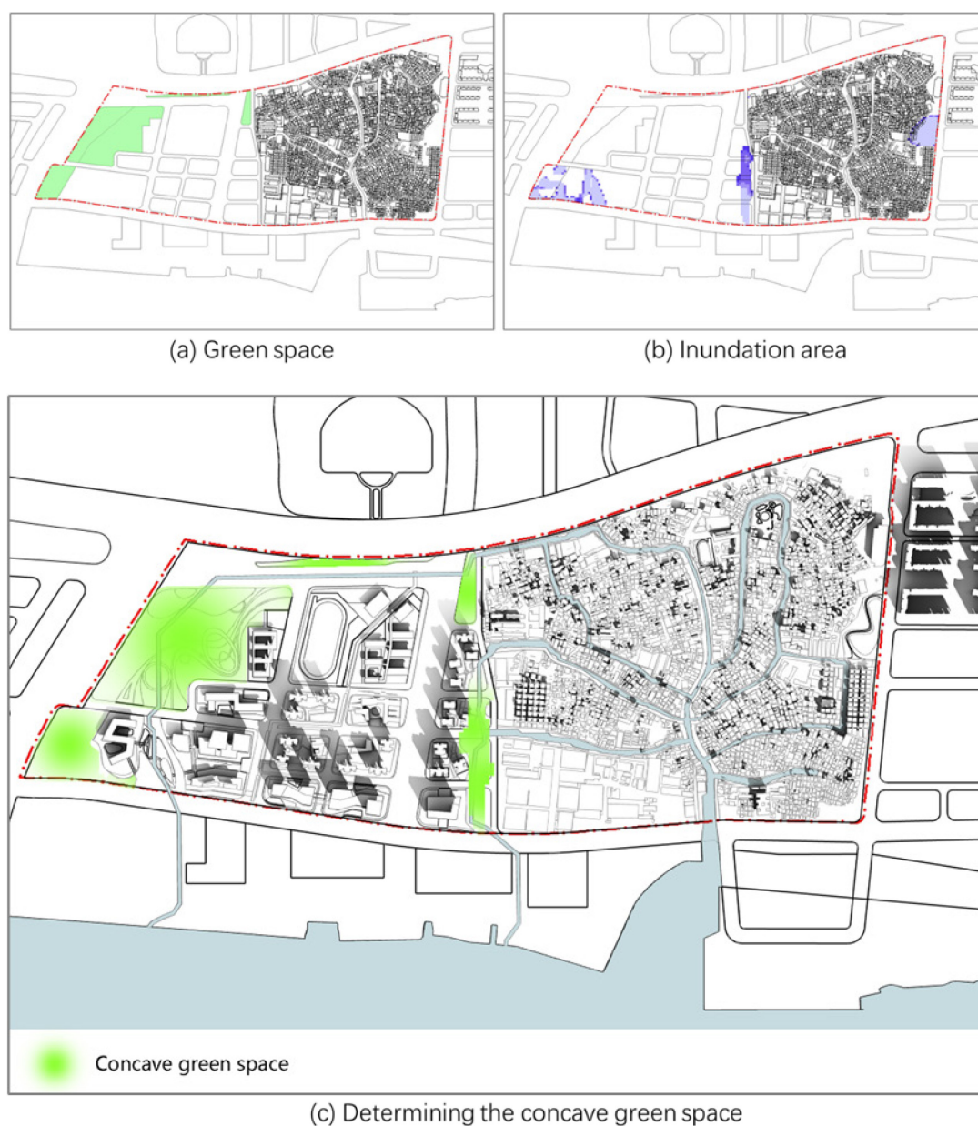
Figure 6-14 Layout process and results of concave green space
