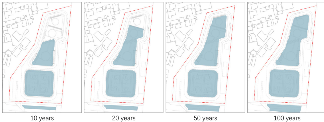
Figure 6-54 Simulation of inundation states under four return periods
