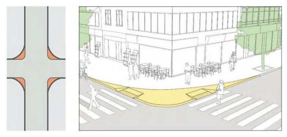
Fig. 4-11 Narrowing intersections to implement small turning radii(Source: Global Street Design Guide)
