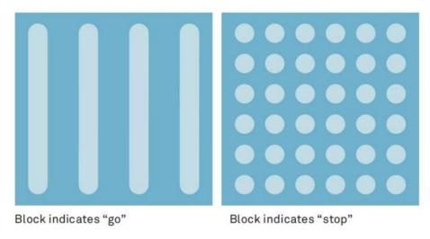
Fig. 4-6 Block indicates "go" and block indicates "stop" (Source: Global Street Design Guide)
