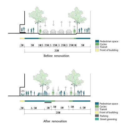
Fig. 6-35 Compressed lane width on Tianhe Nanyi Road to release street space (Source: Completed by author)
