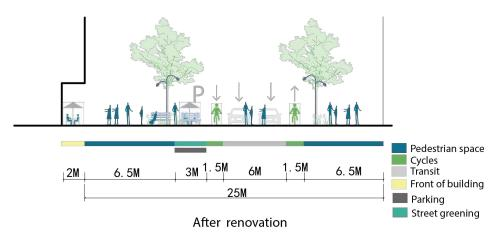
Fig. 6-14 Section of Tianhe Nanyi Road before and after renovation(TeeMall part) (Source: Completed by author)
