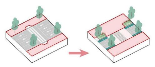
Narrowing of the road surface by widening the pavement
