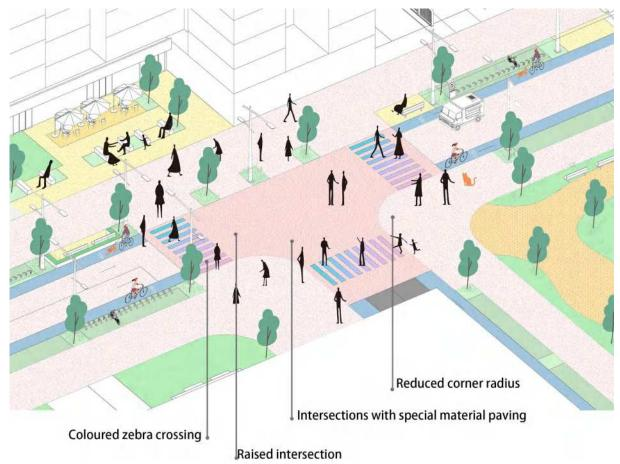
Fig. 6-39 Axonometric view of intersection the street. (Source: Completed by author)
