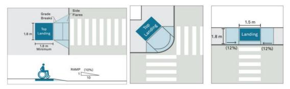
Fig. 4-7 Diagram of Pedestrian Ramps(Source: Global Street Design Guide)
