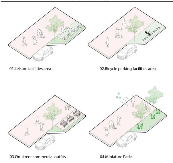
Fig. 6-37 Integrated design of motor vehicle parking spaces and pavement facility zones(Source: Completed by author)
