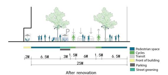
Fig. 6-18 Section of Tianhe Nanyi Road before and after renovation(Parc Central part) (Source: Completed by author)
