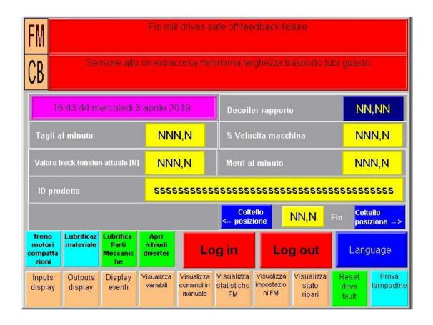
Figure 182. PLC screen example for parameters setup
